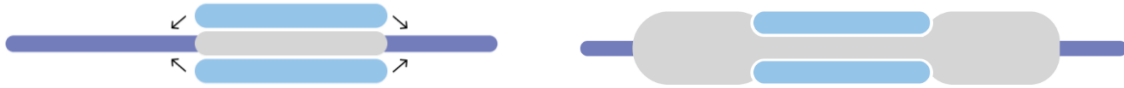
FIGURE 32: CROSS SECTION OF THE SENSOR'S OLD DESIGN (LEFT), CROSS SECTION OF THE SENSOR'S NEW DESIGN (RIGHT)
