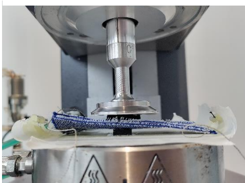
FIGURE 23: WOVEN SENSOR UNDER PRESSURE FOOT OF THE RHEOMETER
