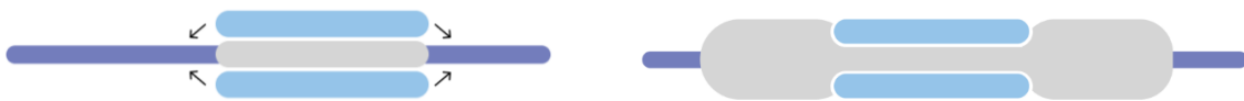
FIGURE 59: SIMPLIFIED CROSS SECTION OF WOVEN SENSOR OLD DESIGN (LEFT) AND IMPROVED DESIGN (RIGHT)
