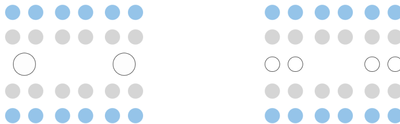
FIGURE 39: CROSS SECTION OF WEFT YARNS, OLD COMPOSITION (LEFT) AND NEW COMPOSITION (RIGHT)
