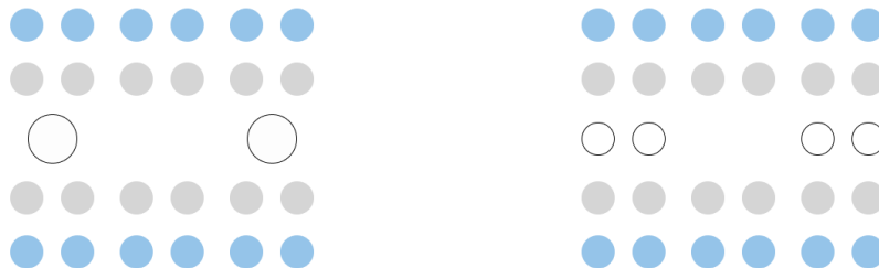
FIGURE 62: CROSS SECTION OF WEFT YARNS, OLD COMPOSITION (LEFT) AND NEW COMPOSITION (RIGHT)
