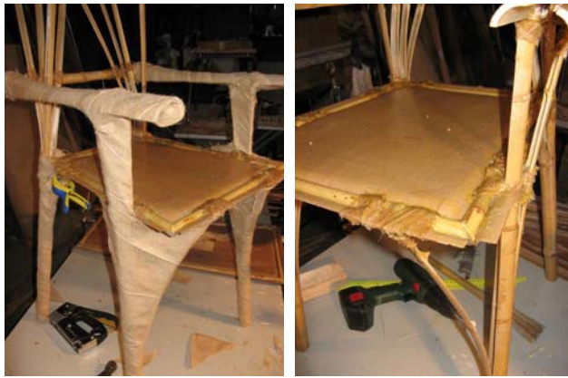
Figure 6.5: Joints developed by Daan van Rooijen consisting of bamboo stems split at the end, wrapped with jute fibers
