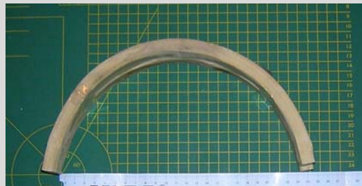
Figure 2.5: bamboo strips curved after steaming procedure
