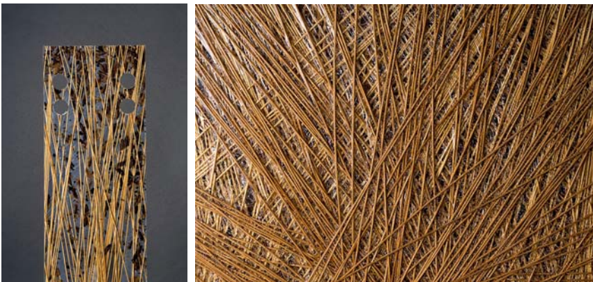
Figure 6.19: Casting the bamboo fiber in the form of small sticks in a transparent resin provides interesting visual effects, such as these samples developed by Ro Koster & Ad Kil (left) and Daan van Rooijen (right) demonstrate
