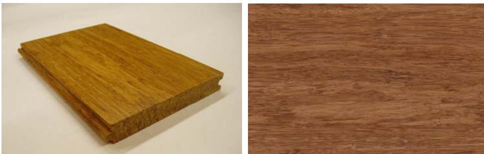
Figure 5.16: Samples of Strand Woven Bamboo (SWB)
