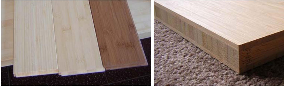
Figure 5.1: Plybamboo is available in various colors, textures and sizes; in the left picture Plybamboo flooring (from left to right: bleached side pressed, bleached plain pressed and carbonized plain pressed) is depicted, in the right picture a sample of a 3-layer carbonized Plybamboo panel is shown
