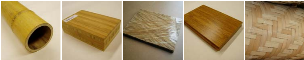
Figure 2.14: Samples of the various bamboo materials used in the final prototypes of the participating designers (from left to right): I) the stem, II) Plybamboo, III) bamboo fiber based composite, IV) SWB, and V) mats
