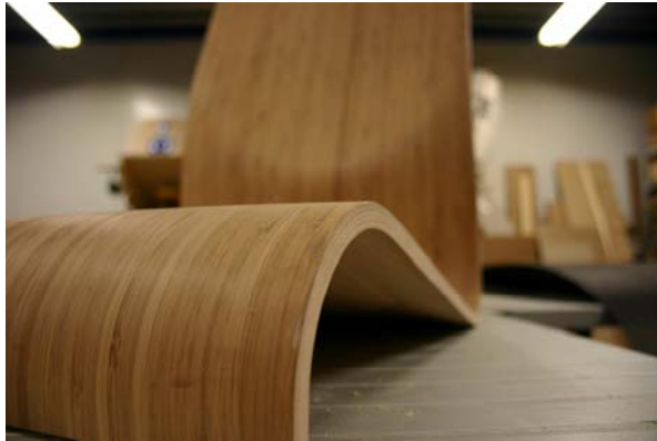
Figure 6.11: Sample of a bended seating at Moso International made from several layers Plybamboo veneer
