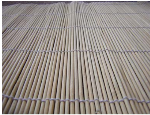
Figure 6.18: Small bamboo sticks commonly used for blinds can also be used in composite materials
