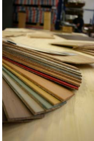
Figure 9.10: Samples of taped mats developed by Moso International, which combine the advantages of bamboo and carpet
