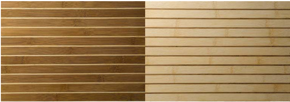
Figure 6.14: New flooring/board material designed by Patrick Kruithof, taking advantage of clean edges of Plybamboo in its in-lays
