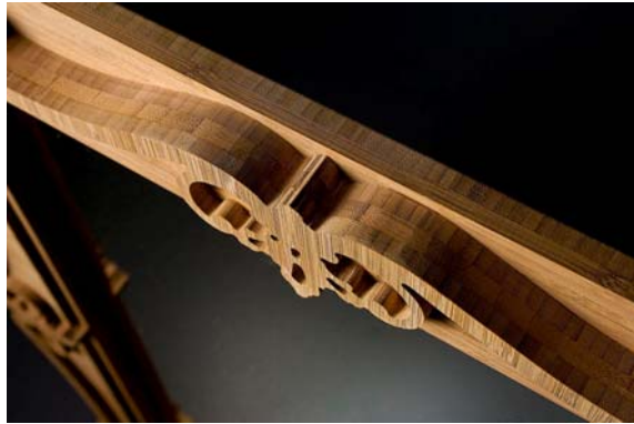
Figure 6.13: Mette Hoekstra has taken advantage of the multi layered-ness of Plybamboo in the design of her mirror
