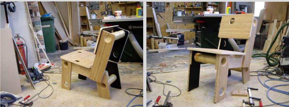
Figure 7.8: Bamboo chair designed by Thijs Bakker, inspired by his design made during the Bamboo Labs, combining the stem and Plybamboo
