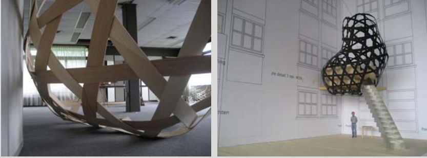
Figure 7.6: Scale model (left) and one-on-one experiment (right) for the coffee corner in the atrium of a school made out of bended Plybamboo by Tejo Remy and René Veenhuizen
