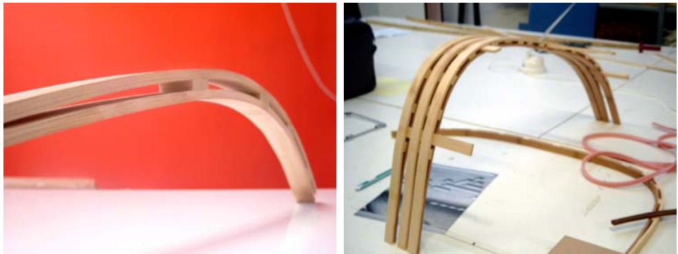
Figure 6.16: Sample of a bending experiment with strips executed by Yvonne Laurysen and Erik Mantel
