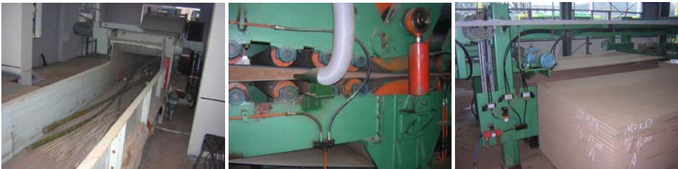
Figure 5.26: Low quality bamboo material used as input (left) for the production (center) of bamboo based MDF (right)
