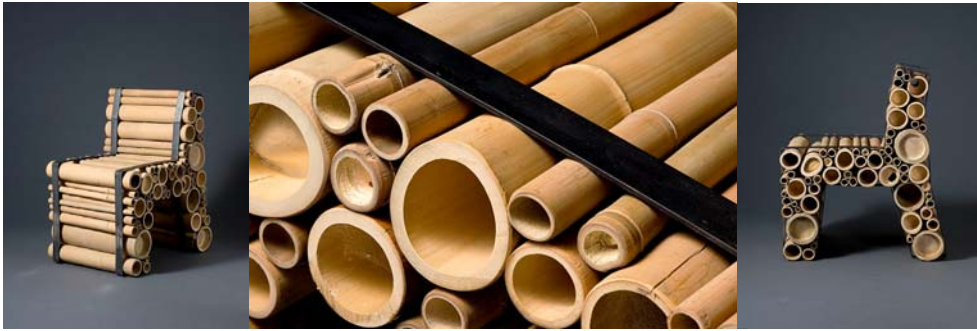
Figure 4.5: Chair by Leonne Cuppen (Yksi) made from the stem Main processing technologies used: sawing and sandblasting
