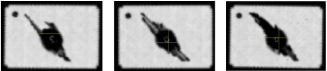
Figure 4.17: C-scans of three TS AP-PLY 2 45° 1/2 specimens impacted at 30 J
