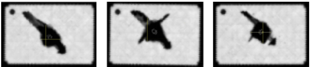
Figure 4.13: C-scans of three alternating AP-PLY 2 90° 1/2 specimens impacted at 30 J
