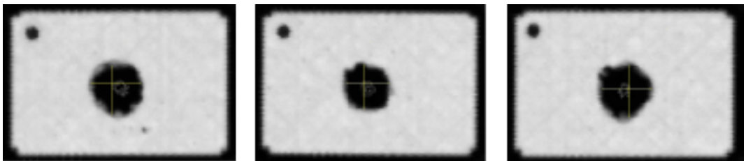
Figure 4.12: C-scans of three AP-PLY 2 90° 1/2 specimens impacted at 30 J
