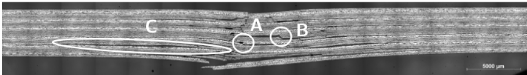
Figure 1.18: Section cut of an impacted specimen
