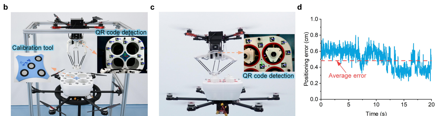
Extended Data Fig. 2 | Onboard vision system of FlyingToolbox. a. The design of the onboard vision system involves six steps: three offline steps (QR code array design, camera calibration, and hand-eye calibration) and three online steps (QR code detection, 6D pose estimation, and filtering at 50 Hz). b. Offline hand-eye calibration was performed using a motion capture system to determine the transformation between the camera frame and the manipulator
