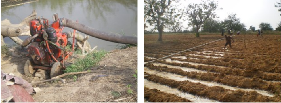
Figure 5.5: a) Diesel pump abstracting water from river b) method of transporting and applying water under riverine irrigation technology.
