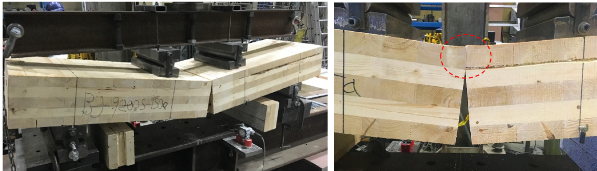
(a) Typical failure modes for BJ specimens
