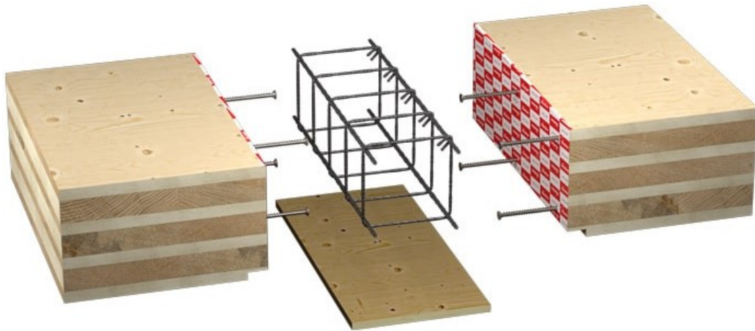
Figure J.1: The concept of the TC FUSION connection [51]
