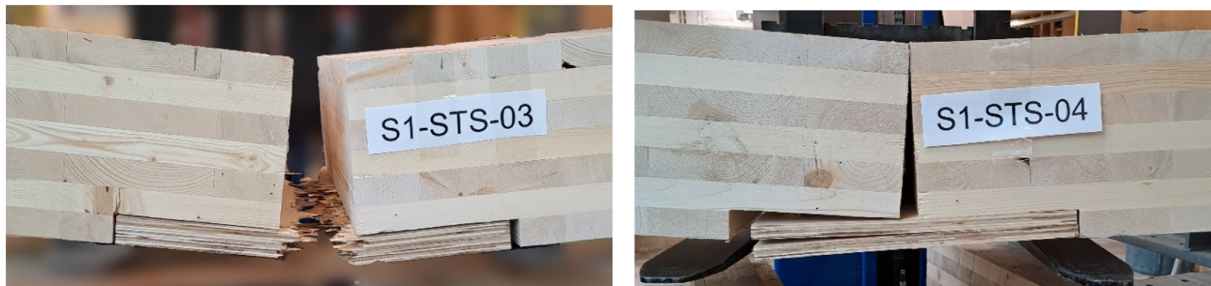
Figure C.3: Failure modes for S1: (a) plywood tension failure; (b) screw withdrawal [30]
