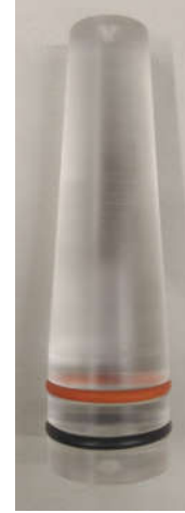
Figure 2.4: Cone used for dye concentration test.
