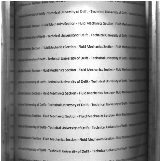
(a) Camera is focused to the tube front resulting in the rear to be blurred.
