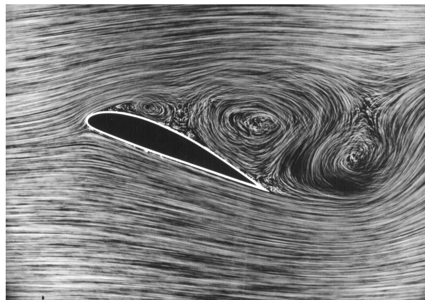
Figure 1.1: Flow separation in action: streamlines stop following the surface and break away (Photo by DLR, 1915) 1
