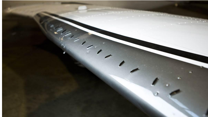
Figure 1.2: Vortex generators on the leading edge of an aircraft wing 2
