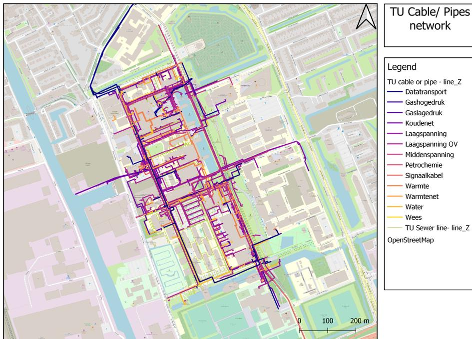
Figure 8: TU cable/ pipes network
