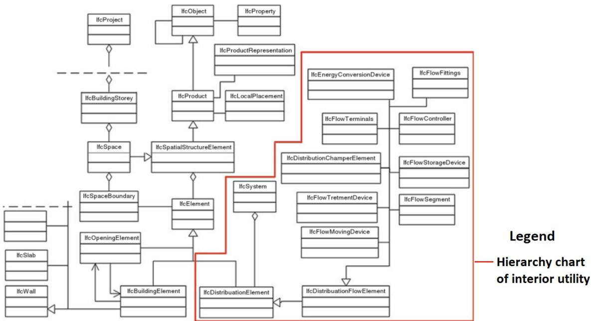
Figure 3: IFC inside building utility network schema
