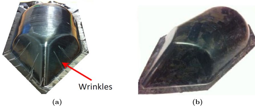
Figure 1.3: Comparison CFC and DFC parts. a) CFC part with wrinkles, [7]. b) DFC part without wrinkles [8]
