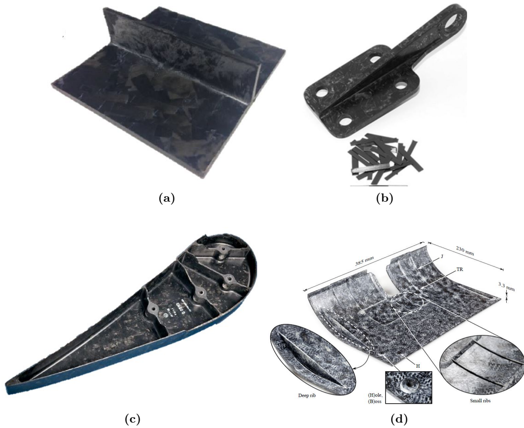
Figure 1.5: Examples of 3D shaped parts made from discontinuous fiber composites a) Rib stiffened structure with inserts [12], b) Door hinge [5], c) T-profile beam [3], d) Demonstrator part of stiffened panel [4]
