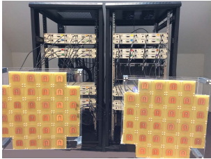
(a) The two distributable 32-antenna arrays in our testbed.
