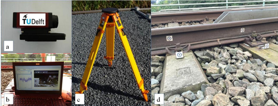
Figure 1.3. Components of the DIC-based device: (a) a high speed camera; (b) processing system; (c) a tripod; (d) targets.
