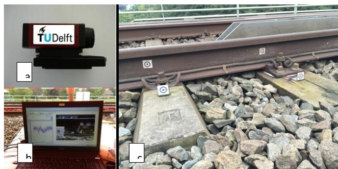
Figure 2.8. DIC-based device: (a) high speed camera, (b) operational system, and (c) targets on rails or sleepers.
