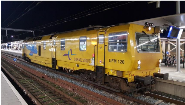
Figure 6.3. EURAILSCOUT UFM120 measuring coach [48].
