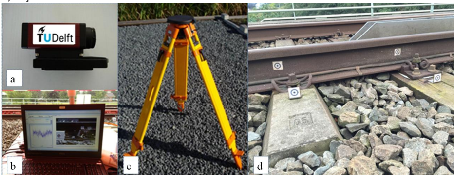
Figure 6.4. A DIC-based device: (a) a high-speed camera; (b) processing system; (c) a tripod; (d) targets.
