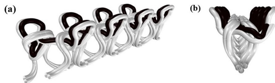
Figure 14. (a) The illustration of the knitted sample which conductive yarn inserted inside and elastic yarn positioned outside (CI), (b) Representation of the unfolded loops in a course which shows the relative position of the conductive (black line) and elastic (grey line) yarns.
