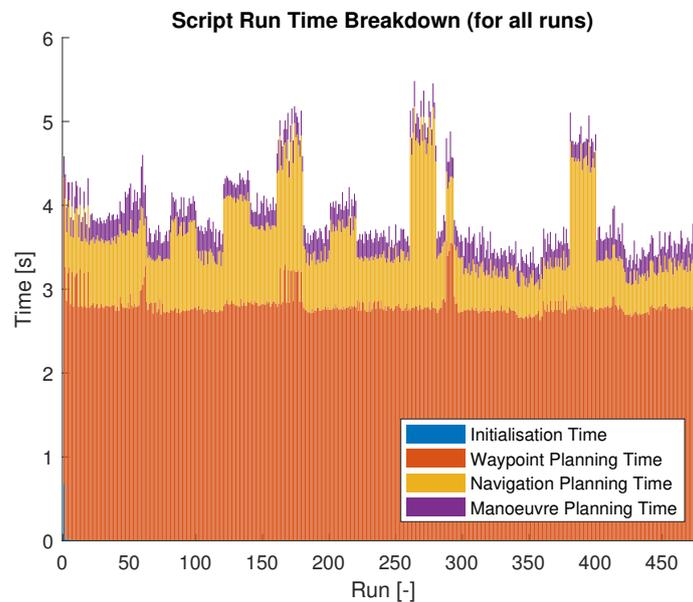
**Figure 4-6:** Script run time breakdown into initialisation, waypoint planning, navigation planning and manoeuvre planning. The initialisation time is so small it is not visible in the Figure.
