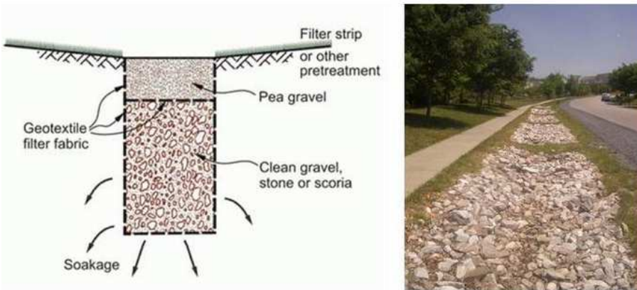
Figure D.26: Example infiltration trench (SSWM, 2015).
