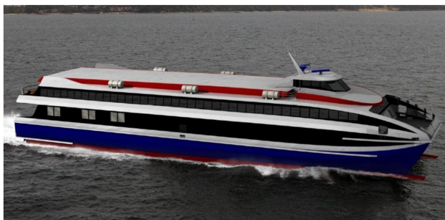
figure 4.1 – the Damen Fast Ropax 6016, dimensions: 60x16.2x2.0 m 3 , maximum speed: 35.0 kn capacity: 660 passengers and 49 cars
