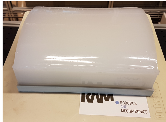
Figure 8.12: Thigh phantom made of silicone rubber.
