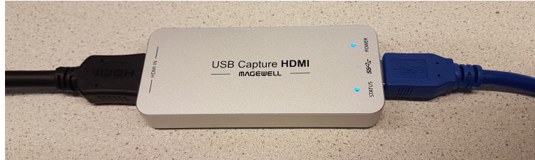
Figure 8.5: Magewell USB Capture HDMI Gen 2 device for transferring ultrasound images from the ultrasound system to the Linux PC.
