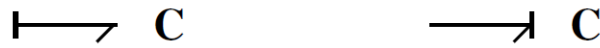
Figure B.2: C element in integral form (left) and in differential form (right) [42].
