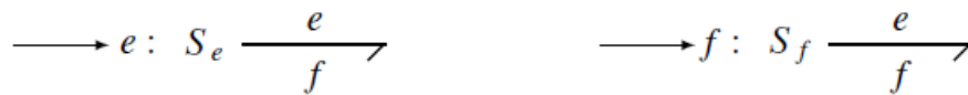
Figure B.7: Bond graph representation of an effort source element (left) and a flow source element (right) [42].
