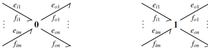
Figure B.8: Bond graph representation of a 0 -junction (left) and a 1 -junction (right) [42].
