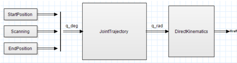
Figure 10.2: Building blocks of the trajectory generator.
