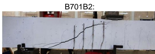
Figure 101 Case B701B2: experimental flexural shear failure
