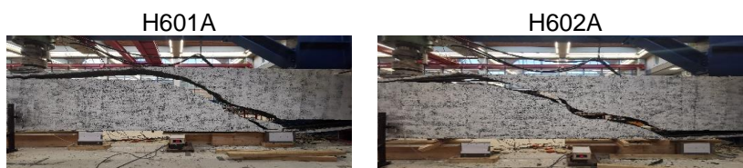
Figure 103 Case H601A: experimental flexural shear failure
