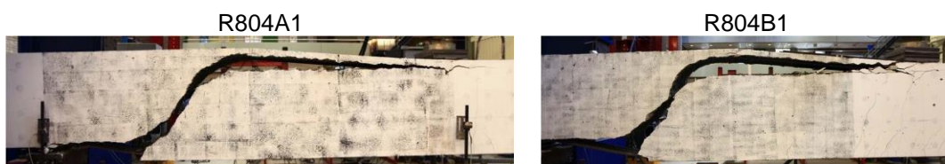
Figure 102 Case R804A1: experimental flexural shear failure
