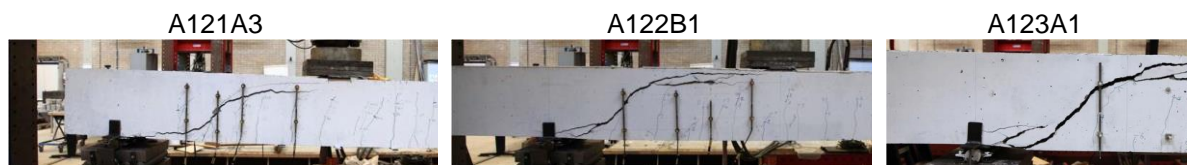
Figure 100 Case A121A3: experimental flexural shear failure
