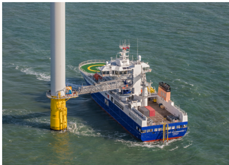
Figure 8.9: W2W-vessel 'Bibby WaveMaster 1', with motion compensated gangway in operation [1]
