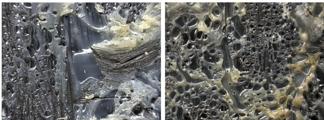
Figure 16 (a) Detail from fracture surface on sample welded at 60 mm/s showing similar porosity to that found in samples on which force was released right after vibration, (b) Detail from fracture surface on regular sample on which force was released right after vibration. Scale bars: 50 \mu\text{m} .
