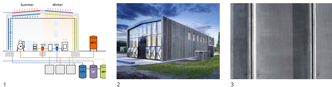
FIG. 3.15 Example of liquid BIST system with seasonal storage (1, 2) in the ETA-Fabrik Factory Prototype and close up of exchange wall (2). Redrawn and photo (Maier et al., 2016).
