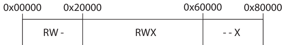
Figure 3.3: Example of the union mechanism for overlapping regions. Two regions are defined, one with read only permission from 0x00000 to 0x60000, and the other with write only permission from 0x20000 to 0x80000. In the overlapping segment the permission becomes the logical sum of permissions: RWX.
