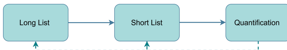
Figure 3.1: Overview of the Methodology: “Three-Stage Rocket”. The methodology is followed from left to right, with the dashed arrows indicating the iterative nature of the methodology.
