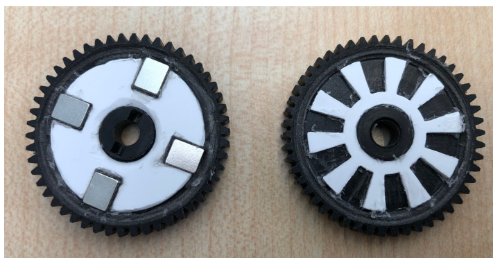
Figure 3.6: Left: One side of the main gear with the 4 Neodymium magnets. Right: White detections are added to the gear for the IR sensor, note that the white ring is not seen by the IR sensor due to the sensor gate.
