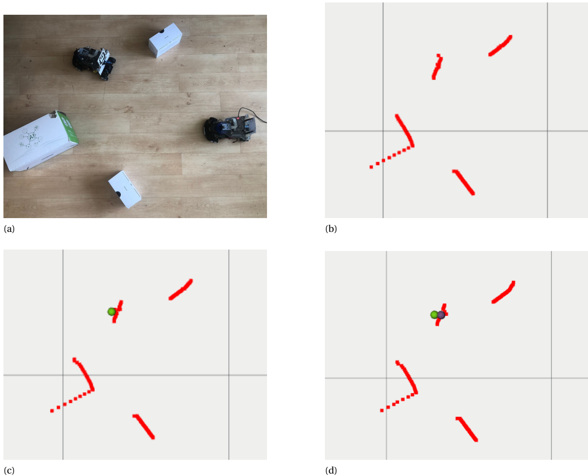
Figure 4.6: Setup of one R2C Car identifying and locating another R2C Car. (a) an image of the setup with (b) the corresponding 2D point cloud. (c) The green point locates the AprilTag tag location. (d) The cluster location with the smallest Euclidean distance to the tag location thus identified the correct location of the R2C Car in the point cloud.
