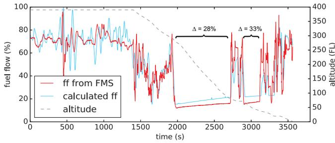
Fig. 2. Original BADA vs FMS fuel flow for Airbus A330-200
