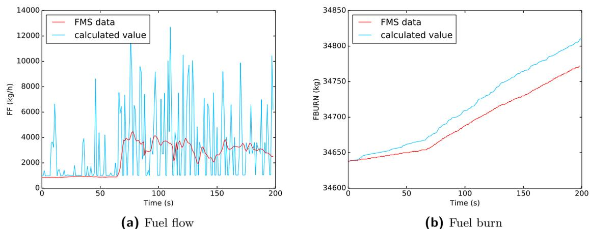
**Figure 4-2:** FMS data vs BADA estimates with finite difference method
