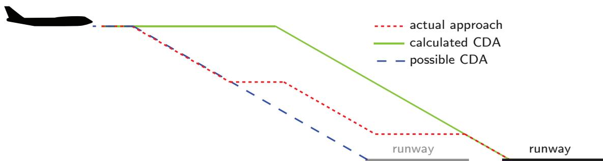
**Figure 3-4:** CDA calculated along the lateral path of the original flight
