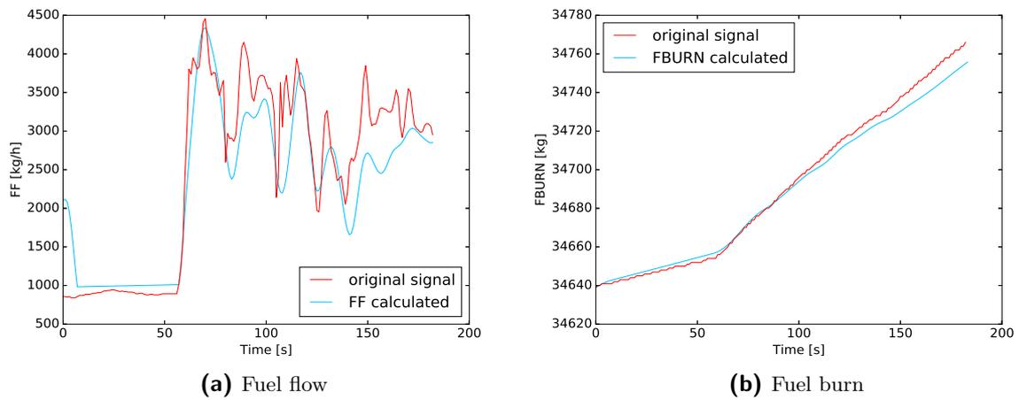
**Figure C-5:** FMS data vs BADA estimates with Gaussian filter sample size four
