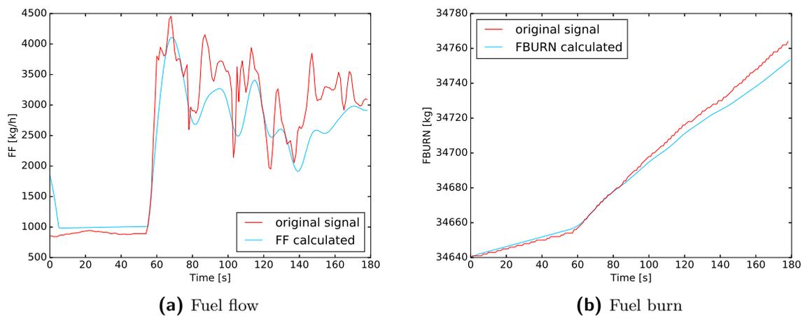
**Figure C-6:** FMS data vs BADA estimates with Gaussian filter sample size five
