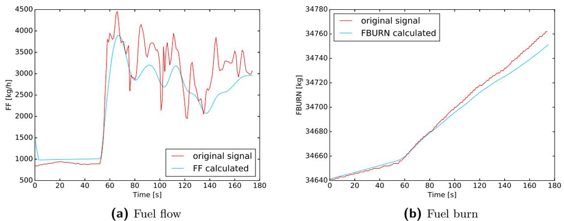
**Figure C-7:** FMS data vs BADA estimates with Gaussian filter sample size six
