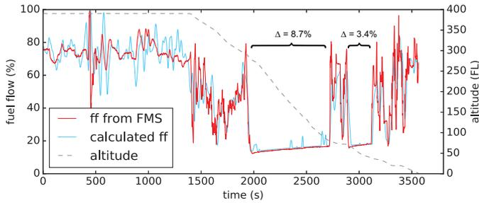
Fig. 3. Calibrated BADA vs FMS fuel flow for Airbus A330-200
