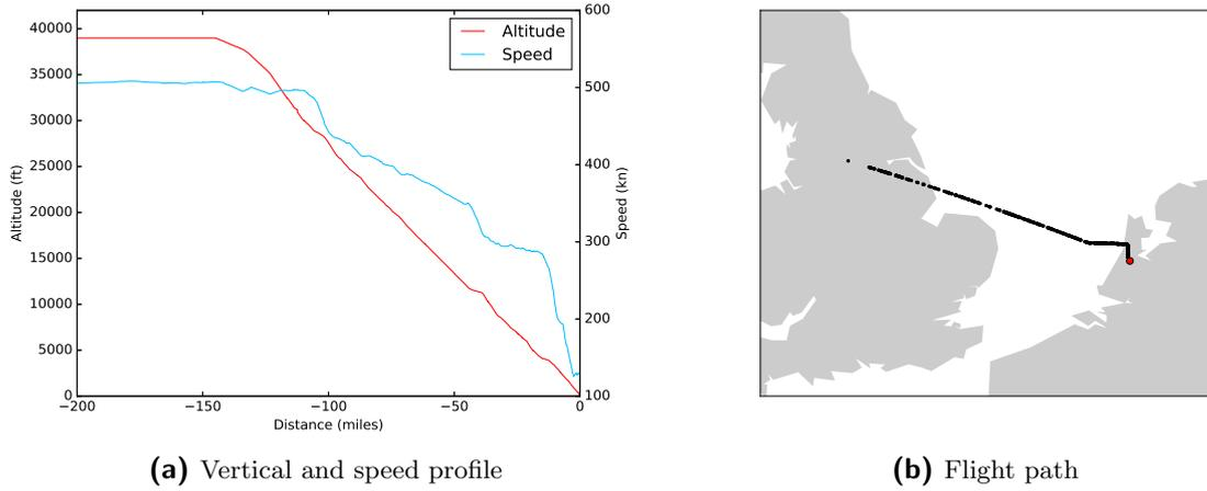
**Figure 4-3:** Example of possible CDA flight of an A330-200
