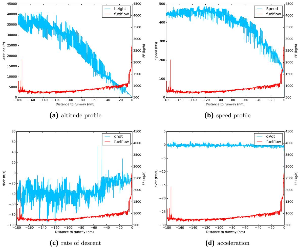
Figure 4-4: CDA profiles for minimal fuel flow
