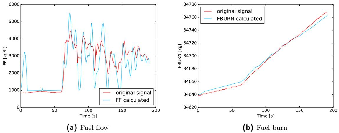
Figure C-3: FMS data vs BADA estimates with Gaussian filter sample size two
