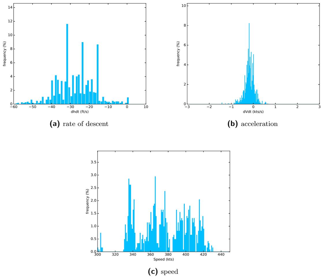
**Figure 4-5:** Most common properties at FL200
