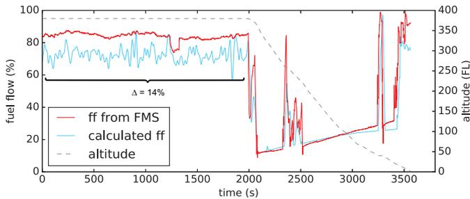
Fig. 4. Original BADA vs FMS fuel flow for Boeing 737-900
