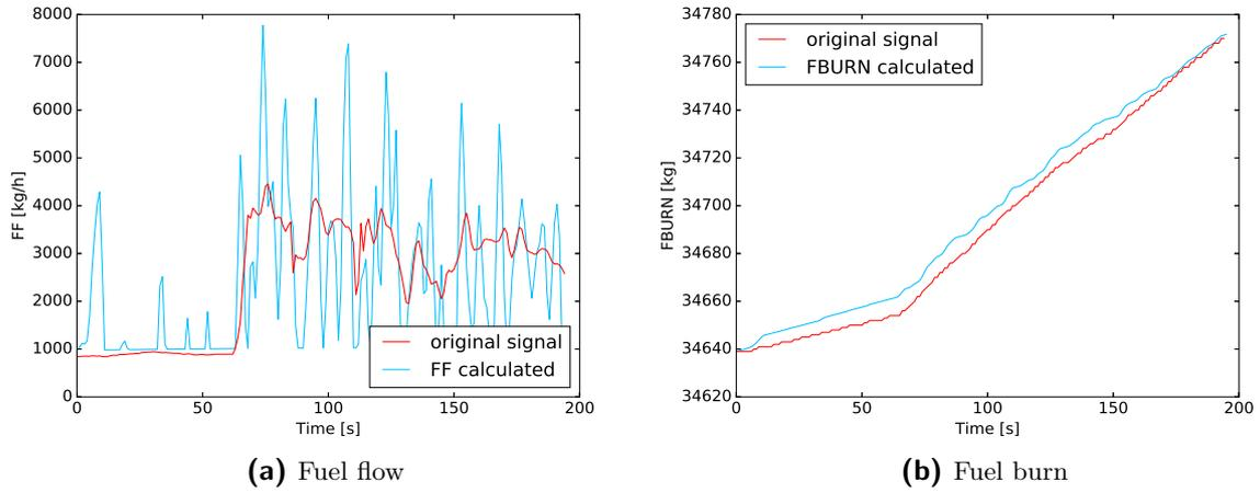
Figure C-2: FMS data vs BADA estimates with Gaussian filter sample size one
