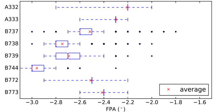
Fig. 10. Fuel-optimal CDA FPAs per FMS a/c type
