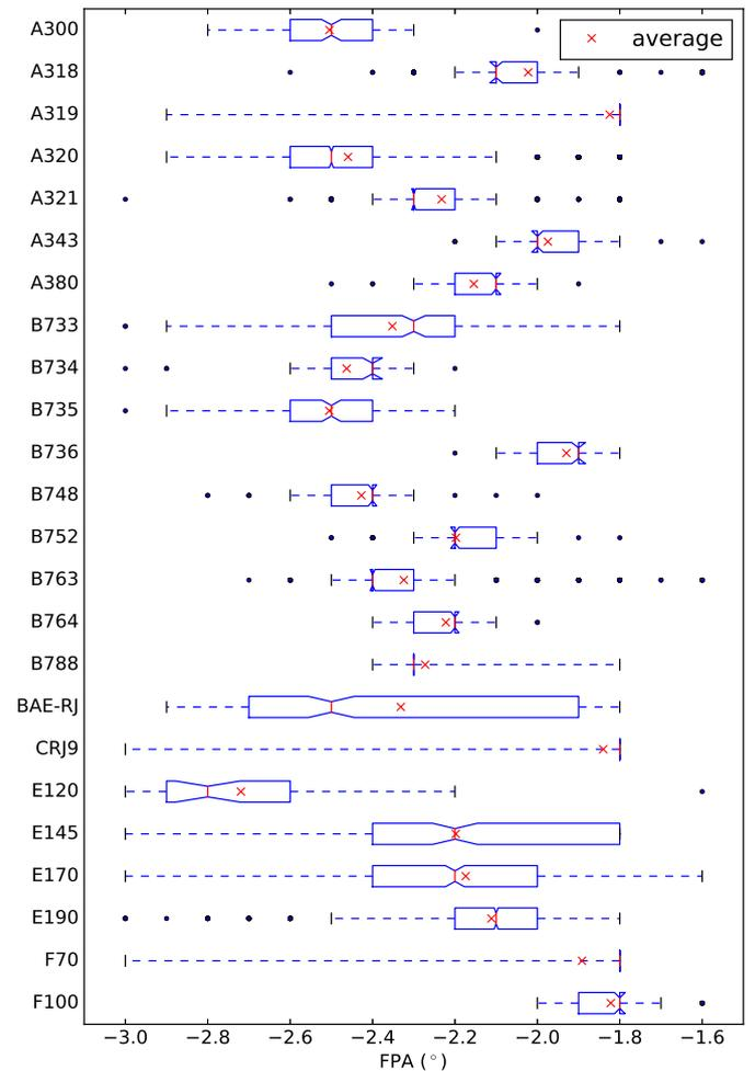
Fig. 11. Fuel-optimal CDA FPAs per ADS-B a/c type
