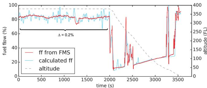
Fig. 5. Calibrated BADA vs FMS fuel flow for Boeing 737-900
