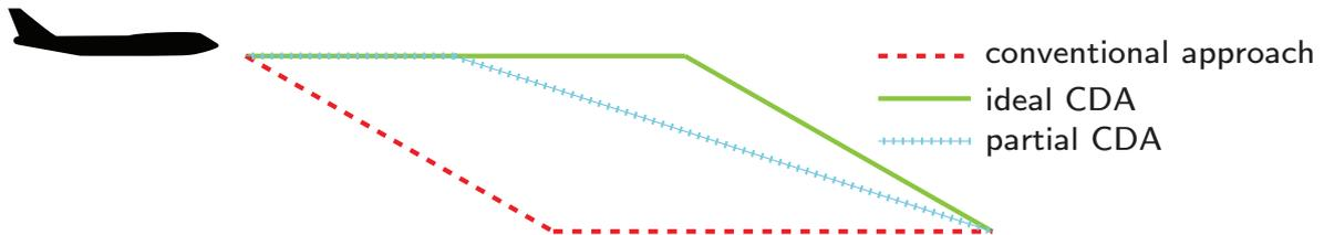
**Figure 2-3:** Possible partial CDA with different thrust settings
