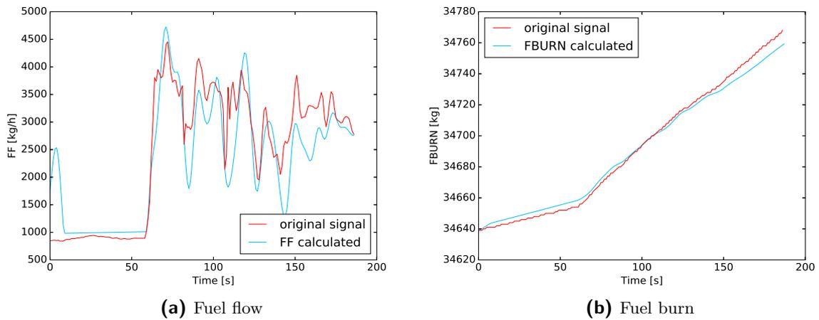
Figure C-4: FMS data vs BADA estimates with Gaussian filter sample size three
