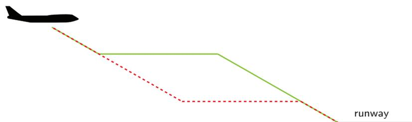
**Figure 2-1:** Horizontal segment at a higher altitude during approach
