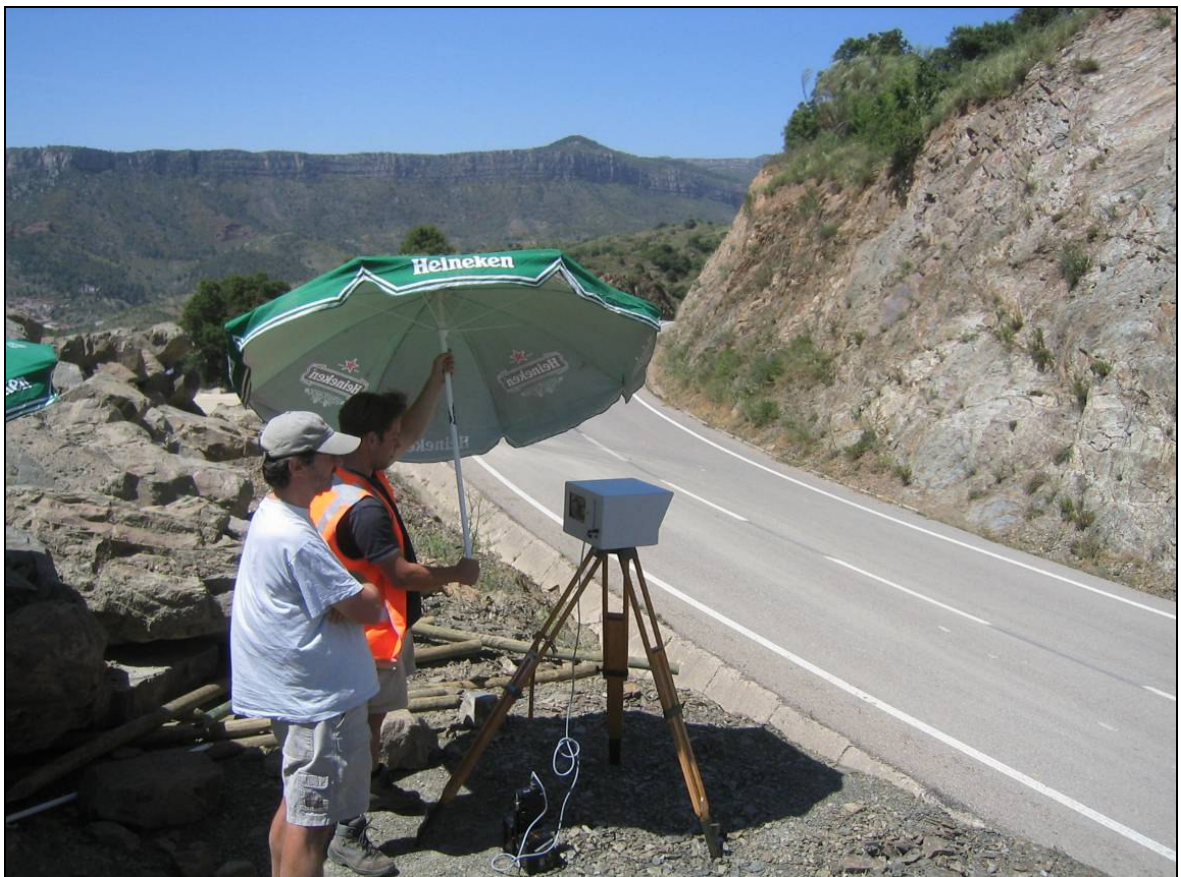
Figure 5.1. Typical laser scanning field survey setup during the field campaign in Spain in June 2004. The laser scanner is an Optech Illris 3-D type. This laser scanner has an external battery pack (on the ground), while the point cloud data is stored on a removable media. The scanner is controlled through the infrared port of a handheld PDA. The umbrella is used to keep the scanner cool and to allow better readings of the LCD control screen on the scanner's back.
