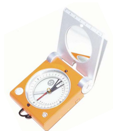
Figure 3.3. Freiburger geologic compass. Developed by Dr. Clar and therefore also referred to as “Clar” compass. This type of compass is mostly used by European geologists.
