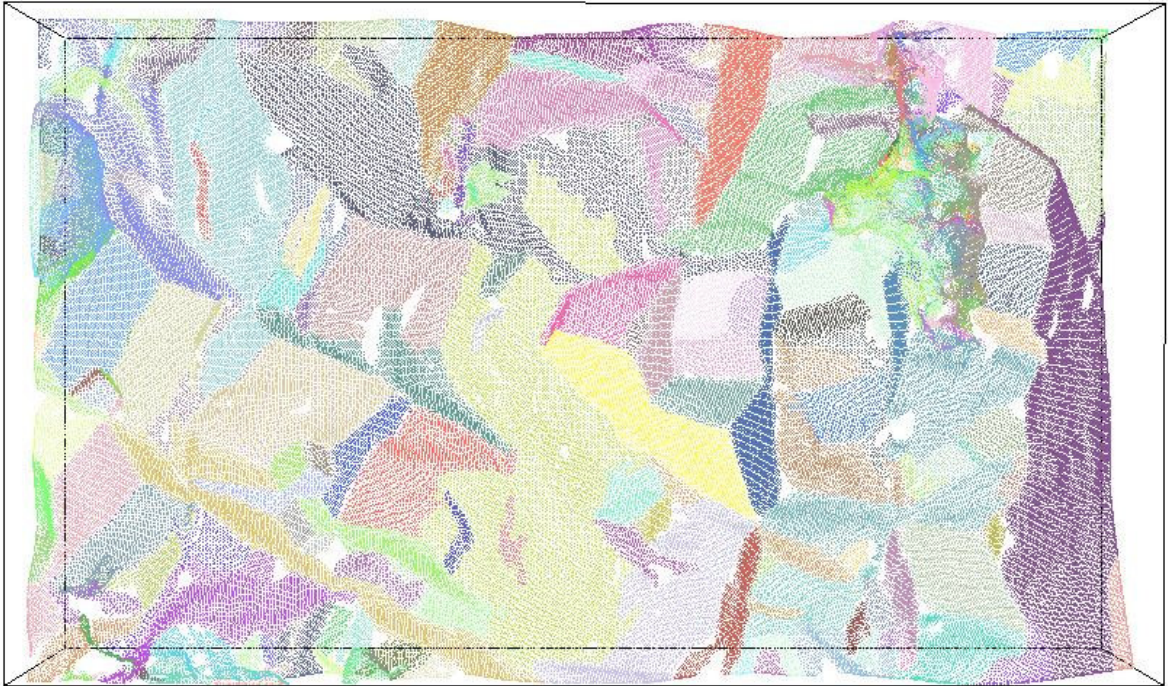
Figure 7.44. This illustration shows the 3-D view of the vertices of the facets from the meshed 3-D surface of Site 2. Note that this is not the laser scan point cloud. Points (vertices) with similar colour represent a single discontinuity plane that is identified with Method 1 (i.e., planes that fall in the same cluster and which are connected are classified to the same plane and receive in this view the same (random) colour).
