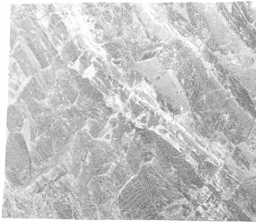
Figure 7.47. The selected point cloud data of Site 1, visualised in a reversed grey-scale based on laser scan intensity. Please refer back to Figure 7.13 for a photograph of the slope where the exact location of this point cloud dataset is outlined.
