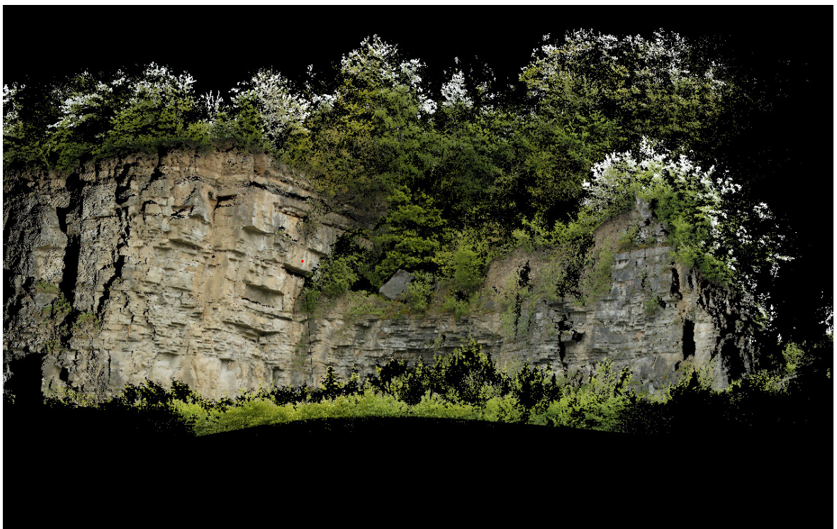
Figure 5.13. Visualisation of the point cloud of the Thon site. Information from the digital camera is used to add colour to the points.
