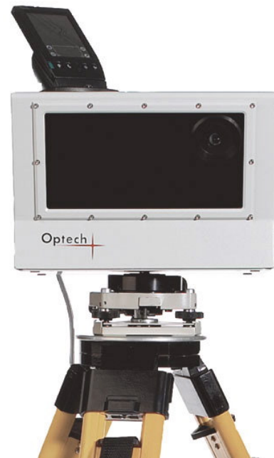
Figure 4.2. Optech Ilris 3-D scanner. On top is the PDA device for operating the scanner. The data is stored internally on a removable memory card.
