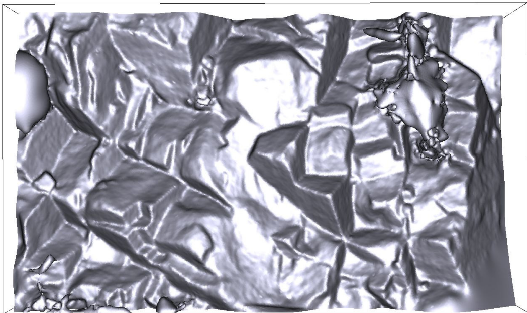
Figure 7.31. 3-D digital rendering of the interpolated and meshed surface that was created with FastRBF. Artificial lighting has been applied to enhance the surface features. The mesh size is 1 cm and the smoothing distance is 2 cm. Note the “blobby” surface in the upper right part of the slope that is caused by vegetation. A large “blob” also appeared in the upper left. This is probably due to a combined noise and edge effect.
