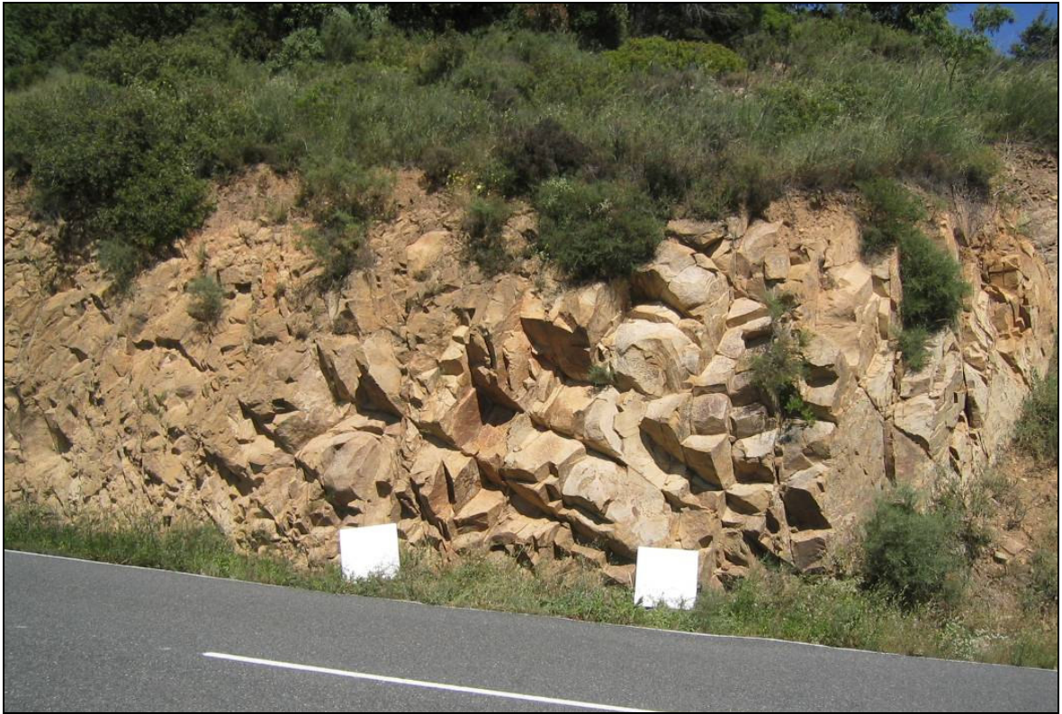
Figure 5.8. Photograph of the surveyed and scanned rock exposure at Site 2. The two white boards act as scale and orientation reference: the left white board has an orientation of 262/70 and the right one 266/70. Both white boards are 60 x 60 cm in dimension. View direction is towards the East.
