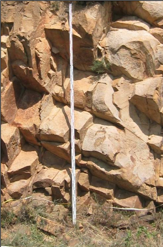
Figure 11.10. Detailed photograph of second vertical scanline (left on the overview picture above).
