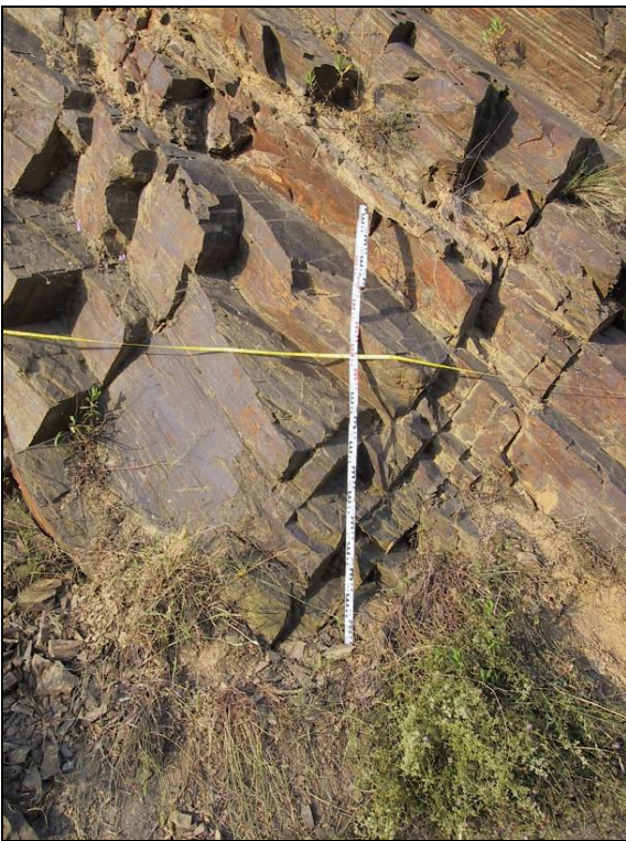
Figure 11.4. Detail of intersection point of horizontal and vertical scanline.
