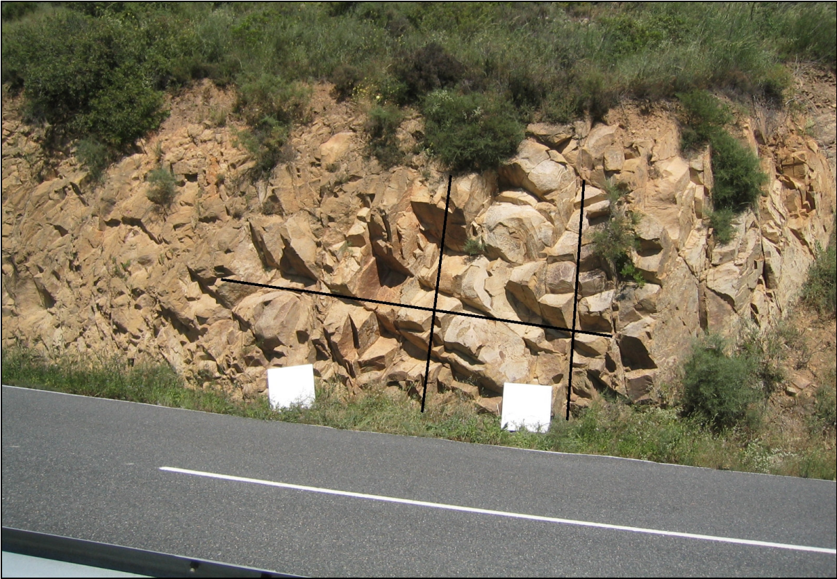
Figure 11.9. Approximate position of the horizontal scanline and the two vertical scanlines near Torroja: Site 2. Scanlines are drawn-in by hand. The horizontal scanline survey was done from left to right over 5.85 metres.
