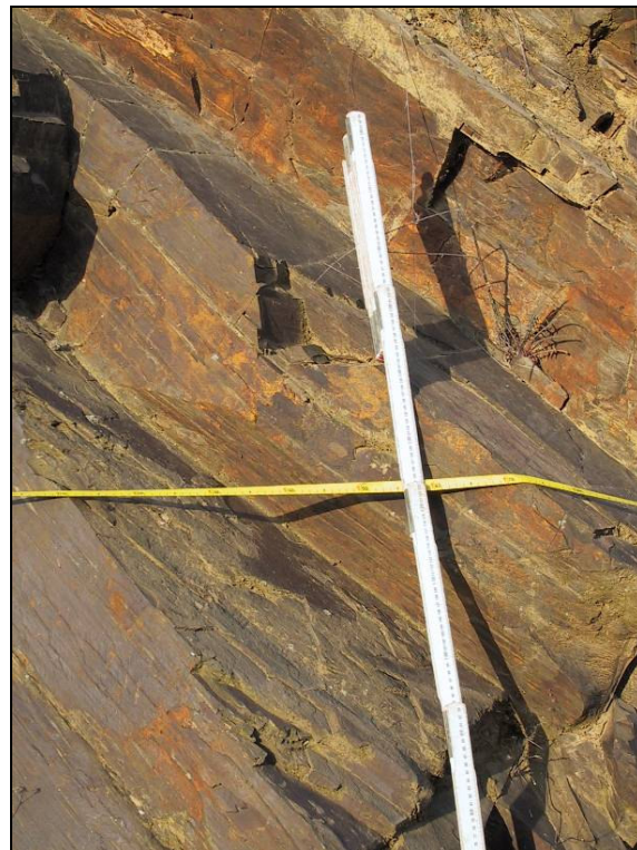
Figure 11.5. More detailed photograph of scanline intersection point, showing the slaty cleavage of the rock mass.
