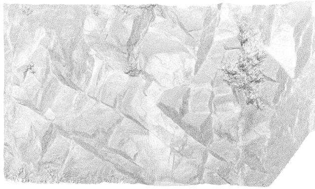
Figure 7.50. The selected point cloud data of Site 2, visualised in a reversed grey-scale based on laser scan intensity. Please refer back to Figure 7.29 for a photograph of the slope where the exact location of this point cloud dataset is outlined.
