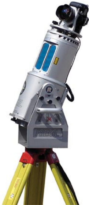
Figure 4.1. Riegl LMS-Z420i scanner with mounted digital camera. In this picture, the scanner is tilted upward. Operation of the scanner is by laptop PC (not shown)
