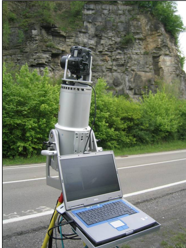
Figure 5.12. Field setup of the Riegl LMS-Z420i at the Thon site. A digital camera is connected with a mount on top of the laser scanner. The camera is geometrically and optically calibrated. This allows the colour information from the digital camera to be added to the point cloud data. The laser scanner is operated by the attached laptop computer.
