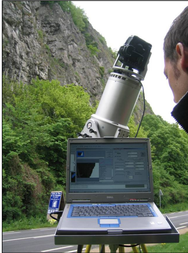
Figure 5.14. Field setup of the Riegl LMS-Z420i at the Dave site. It can be seen that the laser scanner has been tilted backward to obtain an optimal field of view of the upper part of the slope.
