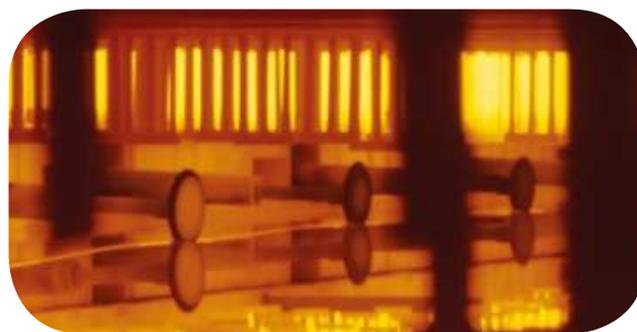
Figure 79. Float tank interior (source: www.cmog.org)
