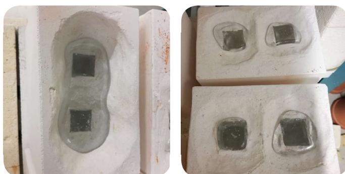
Figure 176. Results after firing (left) mold B where the glass is connected, (right) A molds where the glass is not connected
