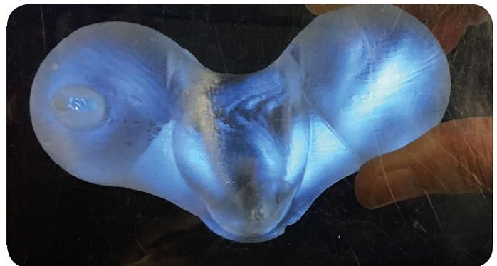
Figure 186. Light-blue isochromatic fringes showing the glass flow of the casting process
