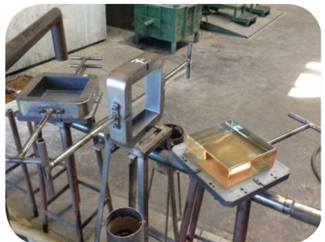
Figure 85. The high precision steel molds used for construction of the Crystal Houses facade (Oikonomopoulou, 2017)
