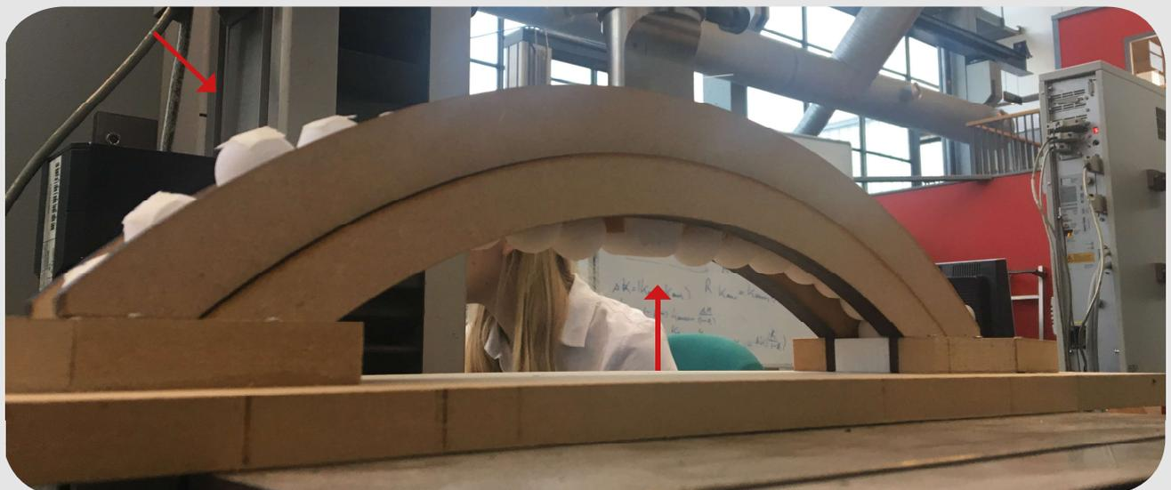
④ Figure 217. Observation of displacement during the test (audible cracks).
