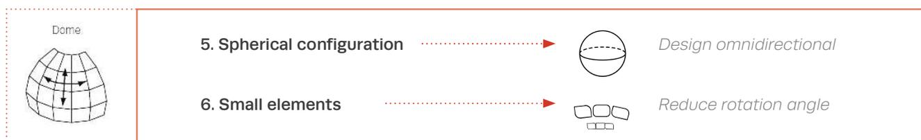
Figure 135. Plus new design principles of cast glass components (double curved structures: domes)
