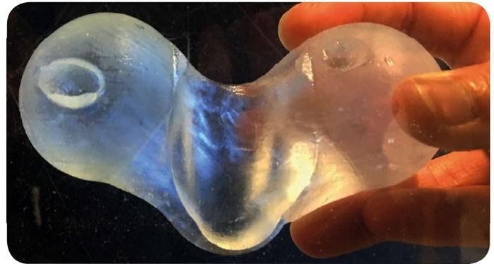
Figure 185. Light-blue isochromatic fringes located at the left top edge
