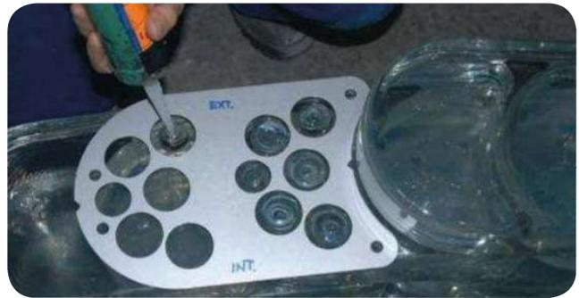
Figure 93. Spacers used for the glue (Göppert et al., 2007)
