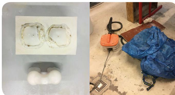
Figure 169. (left) Crystal cast mold with wax model A, (right) water bath with boiler and plastic bags.
