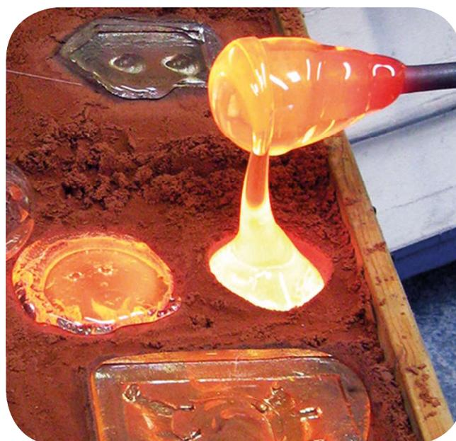
Figure 80. Principle of sand casting
