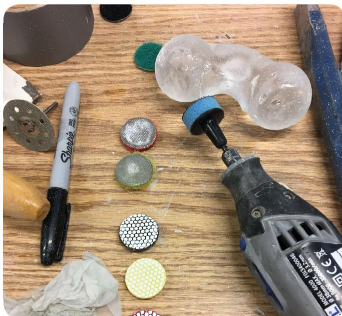
Figure 182. Final polishing of the glass components with the six polishing disc grades.
