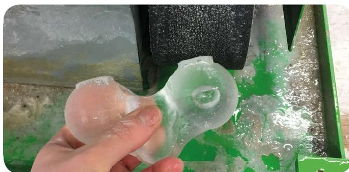
Figure 183. Shaping the funnels to a spherical configuration
