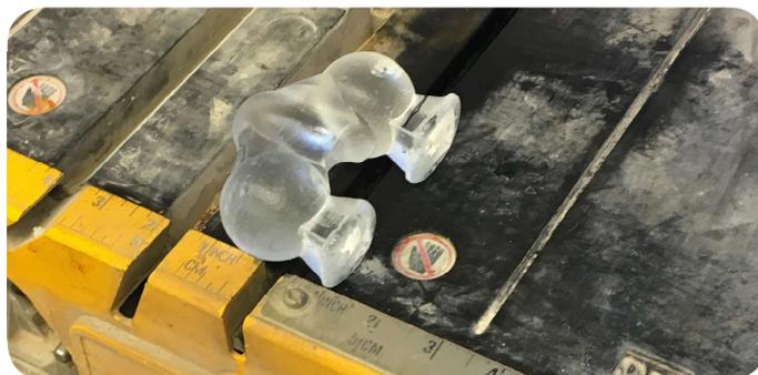
Figure 184. Removing the largest part of the funnels
