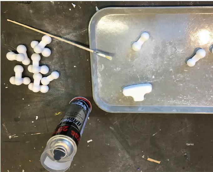
Figure 241. Impregnation of the components
