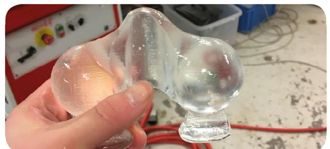
Figure 180. The remaining glass model after the Crystal Cast mold was dissolved
