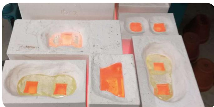
Figure 175. Glowing glass within the molds during firing
