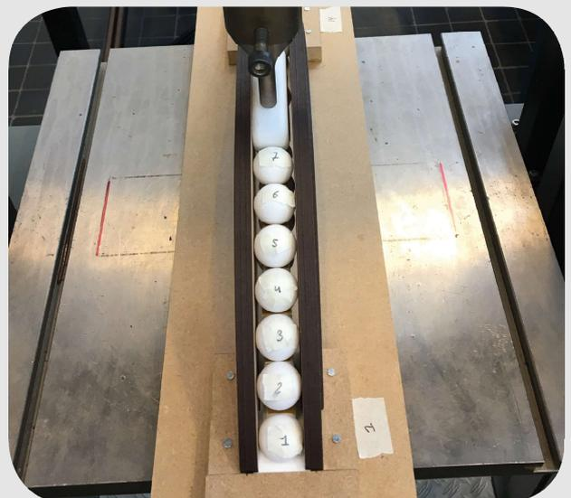
Figure 214. Test set-up physical arch test
