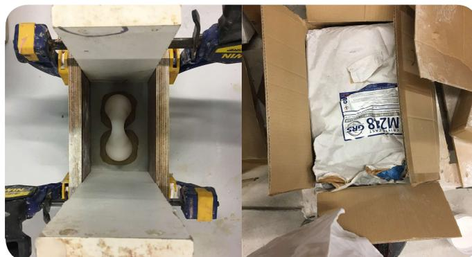
Figure 168. (left) bounding box of mold A, (right) the Crystal Cast M248 powder
