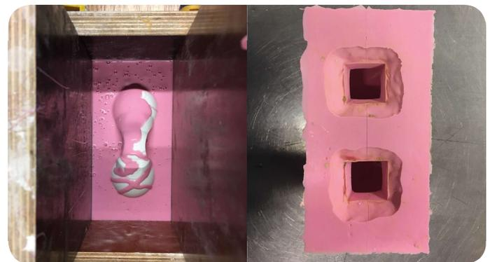
Figure 165. (left) pouring the silicones, (right) silicone mold after curing
