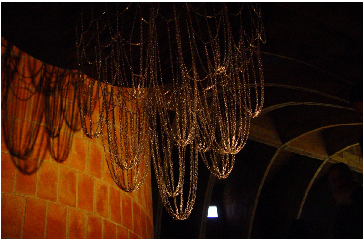
Figure 1.2 Gaudi's catenary model at Casa Milà; Etan J. Tal, Wikipedia.org
