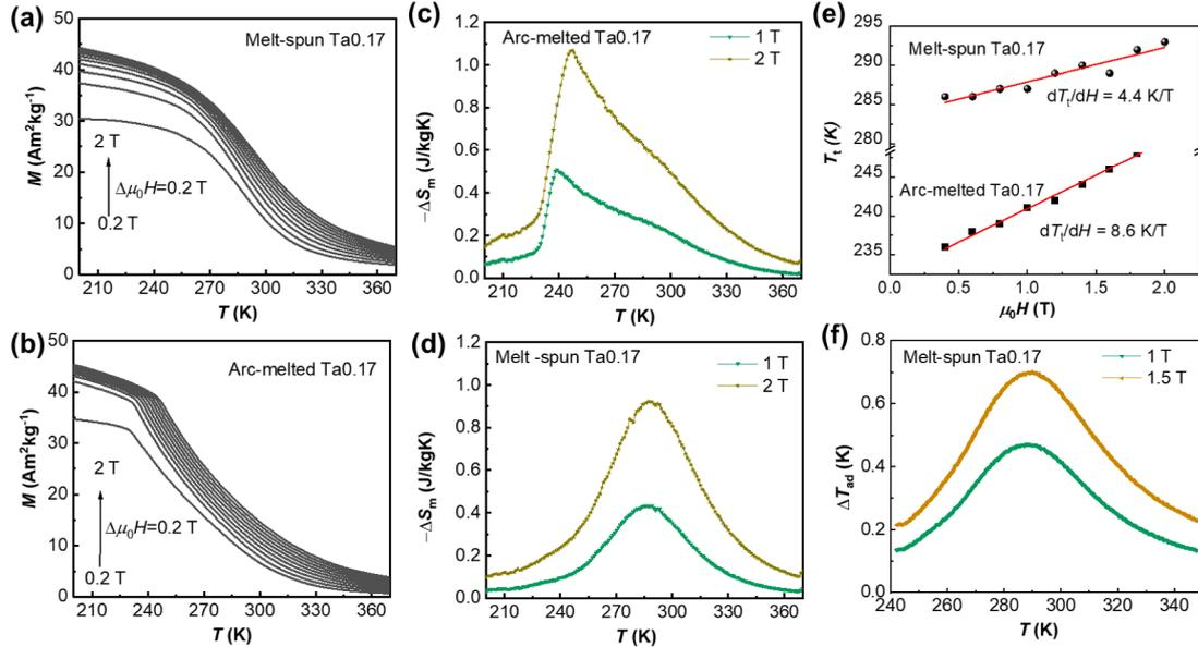
**Fig. 4.**  $M$ - $T$  curves upon heating in different applied magnetic fields for (a) arc-melted Ta0.17 and (b) melt-spun Ta0.17.  $-\Delta S_m$  calculated from the heating curves for (c) arc-melted Ta0.17 and (d) melt-spun Ta0.17. (e)  $T_t$  as a function of magnetic field. (f)  $\Delta T_{ad}$  derived from in-field DSC.
