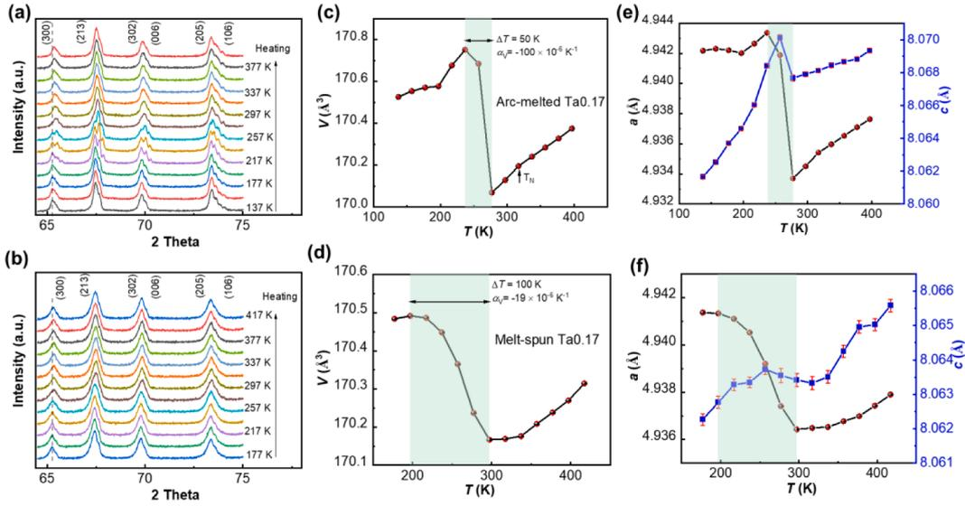
**Fig. 3.** (a, b) XRD patterns as a function of the scattering angle 2 theta, recorded upon heating for a temperature step of 20 K. Temperature dependence of (c, d) unit-cell volume  $V$  and (e, f) lattice parameters  $a$  and  $c$ .
