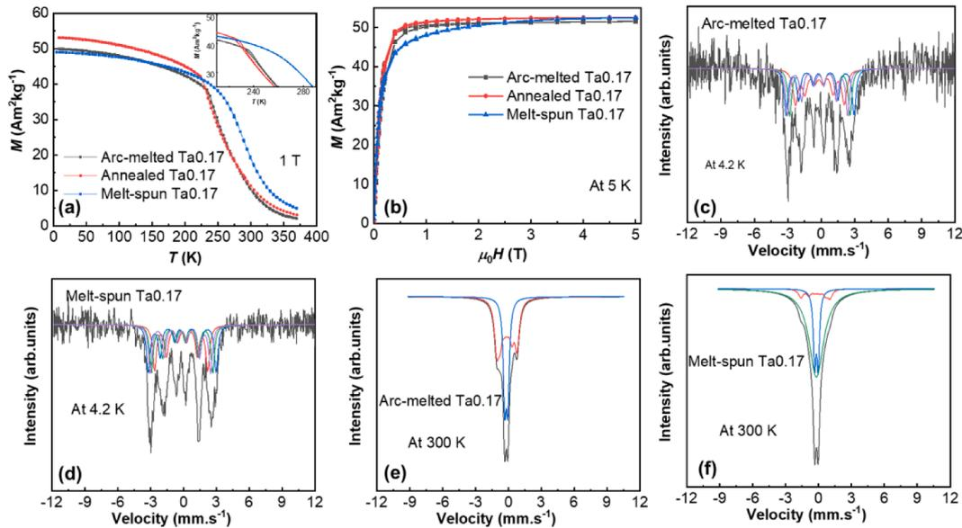
**Fig. 2.** (a)  $M$ - $T$  curves in a magnetic field of 1 T. (b)  $M$ - $\mu_0H$  curves at 5 K. Mössbauer spectra at 4.2 K for (c) arc-melted Ta0.17 and (d) melt-spun Ta0.17. Mössbauer spectra at 300 K for (e) arc-melted Ta0.17 and (f) melt-spun Ta0.17.
