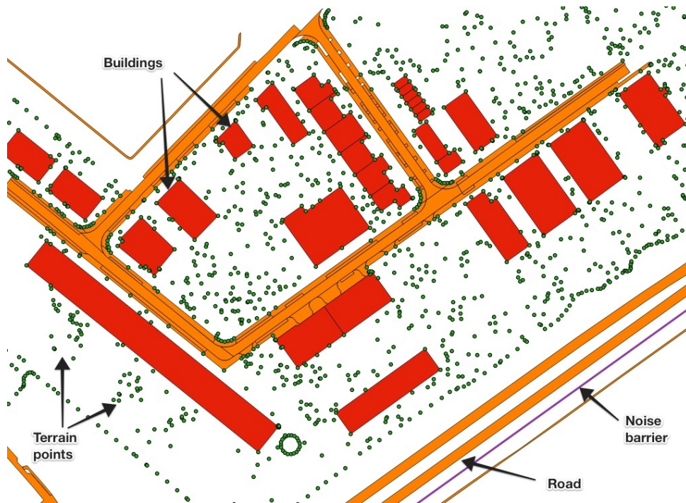
Figure 6: Generated 2.5D input model for road traffic noise
