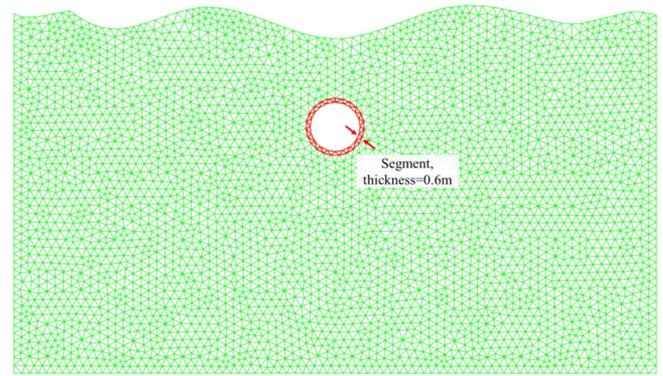
Figure 6. Numerical model for intact rock mass.
