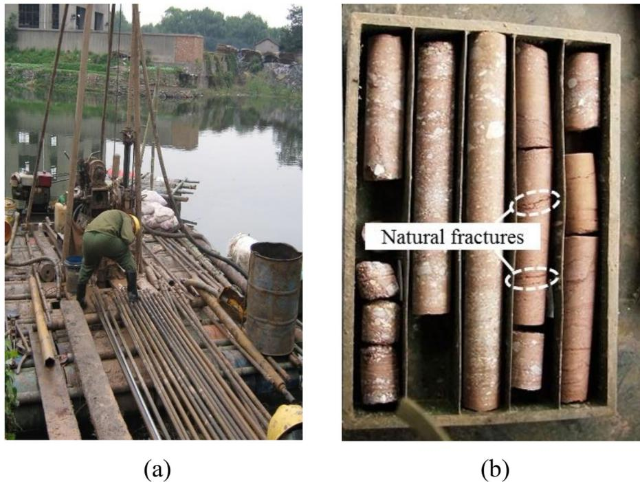
**Figure 2.** Geological exploration in the study site: (a) field environment and apparatus and (b) the rock samples obtained from the site.
