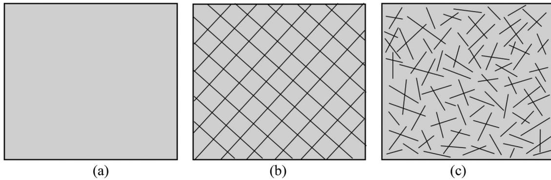
**Figure 3.** The typical conceptual model of different fracture patterns: (a) the original model, (b) the improved model, and (c) the presented random fractures model in this study.
