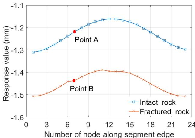
**Figure 10.** The response value of tunnel settlement when the water level changed 1 m.
