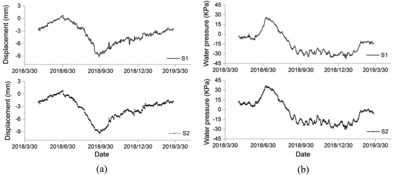
**Figure 12.** The real-time monitoring data obtained from SHMS: (a) displacement of tunnel settlement, and (b) variation of water pressure.
