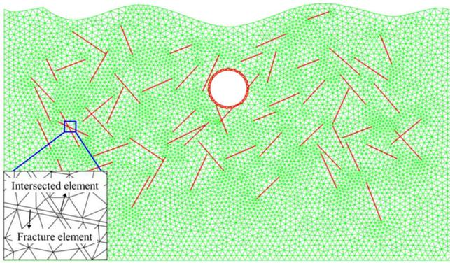
Figure 5. Generation of hybrid elements for the Nanjing Yangtze River tunnel.
