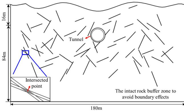
**Figure 4.** Numerical model of fractured surrounding rock in the Nanjing Yangtze River tunnel.
