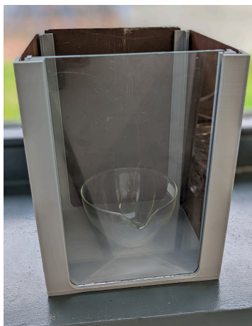
Figure 5.2: First version of the safety chamber. On three sides, a steel plate is used and at the front side a safety glass is used to have a clear view inside the chamber.
