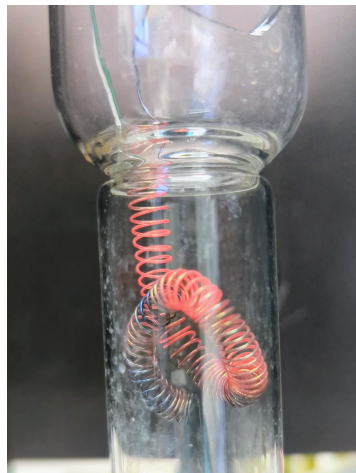
Figure 5.6: Curled heating coil inside the glass tube, to have more space covered with it.
