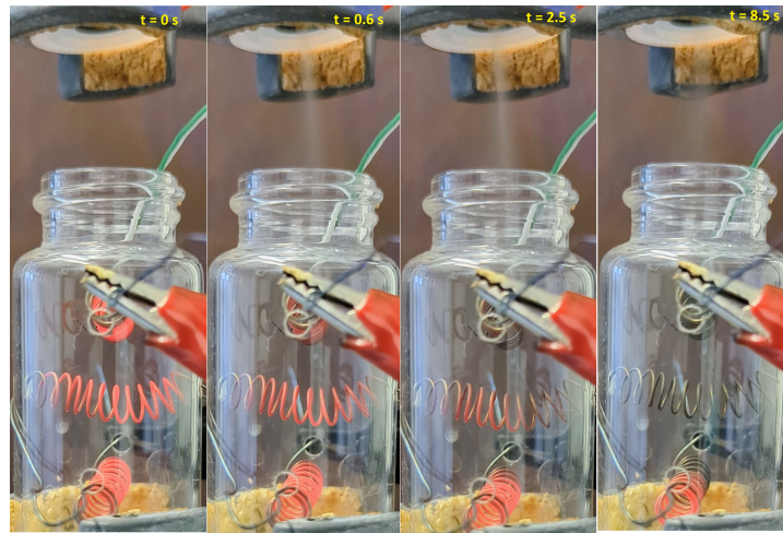
Figure 5.14: Different frames have been taken from a video, which shows how the heating coil is cooling when being in contact with the atomized liquid.
