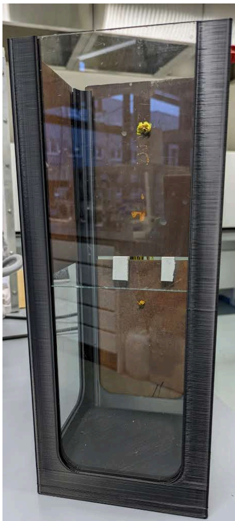
Figure 5.13: Third version of the safety chamber. Compared to the previous version, the bottom part has been raised.
