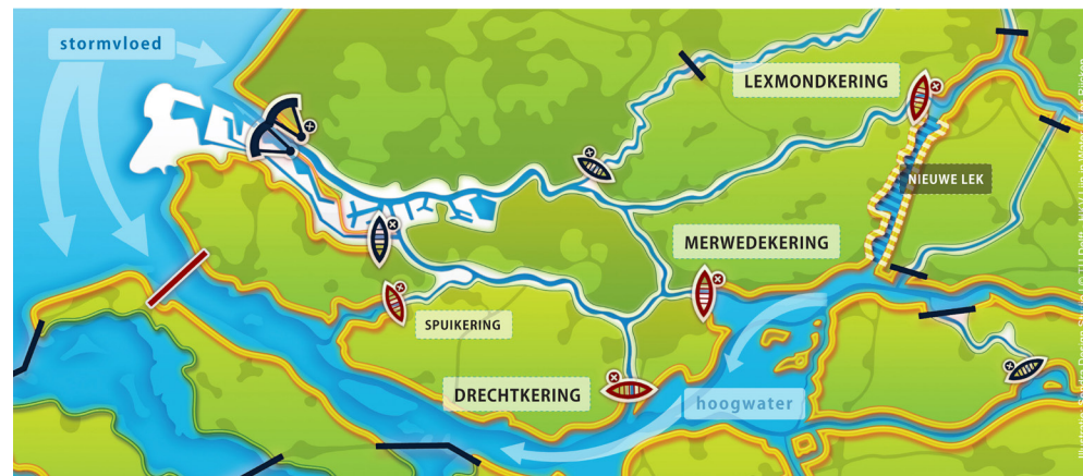
3.35 Four optional river barriers in the tidal rivers and a new river, according to the concept Rhine estuary closable but open (Deltacommittee 2008; Rijcken et al. 2010).
