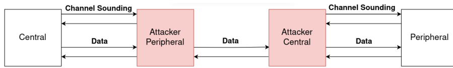
Figure 3.3: Flowchart showing how the attacker can still participate in channel sounding during two-way ranging.
