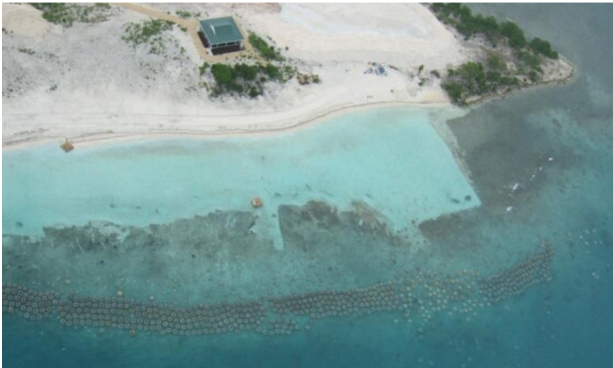
Figure 3.11: Artificial reef made with Reef Balls™ in Antigua
