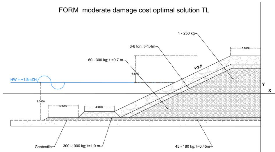
Figure 5.5: Probabilistic cost optimal configuration (FORM)
