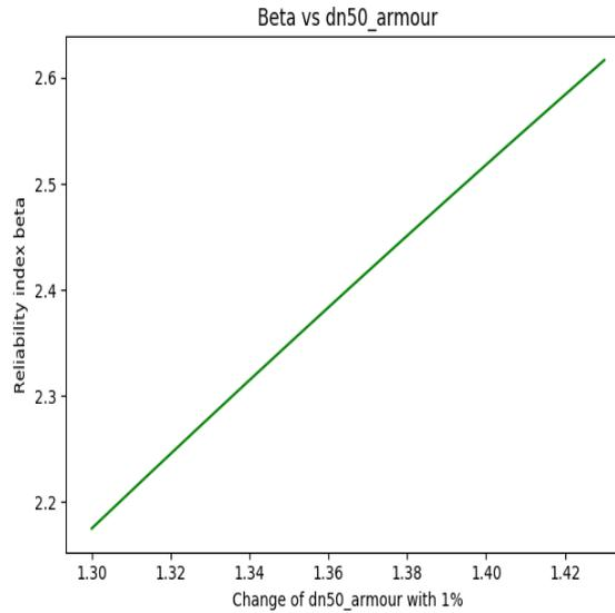
Figure 6.6: Sensitivity of  $dn50_{armour}$  change by 1% to the reliability index  $\beta$
