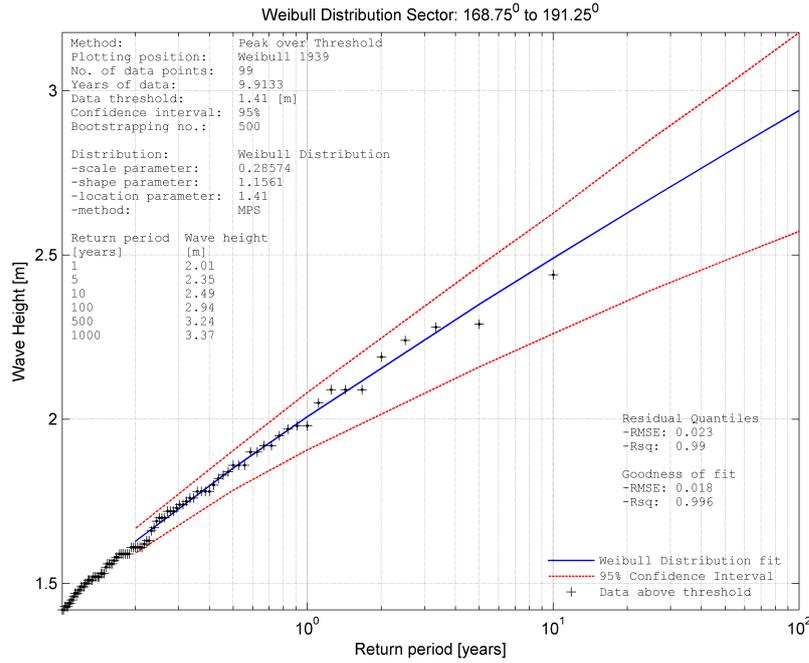
Figure 4.6: Weibull representing the best fit for the extreme significant wave height.
