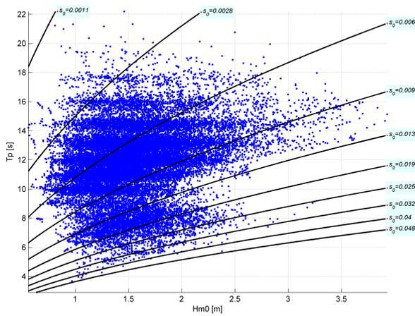
(a) Wave height  $H_s$  versus Wave period  $T_p$  graph with steepness  $s$  lines
