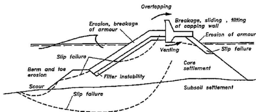
Figure 2.2: An overview of different failure modes of a breakwater (Burchart, 1995)
