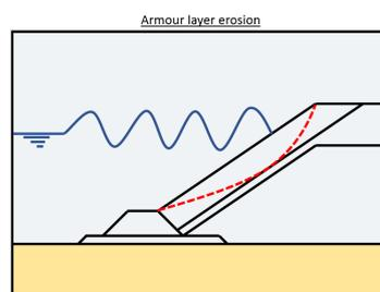
Figure 2.4: Failure Mechanism: Armour layer erosion
