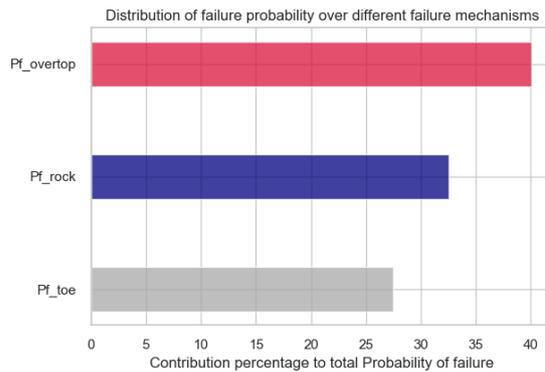
Figure 6.1: Distribution of the probability of failure over different failure mechanisms, initial combination
