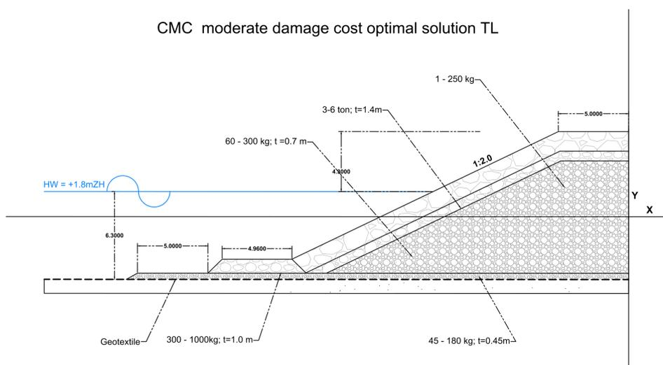
Figure 5.4: Probabilistic cost optimal configuration (CMC)
