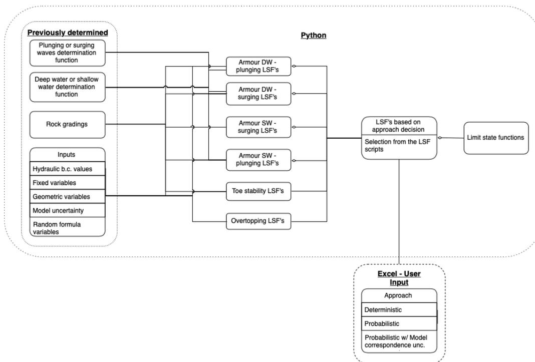
Figure C.5: Model implementation Limit state functions
