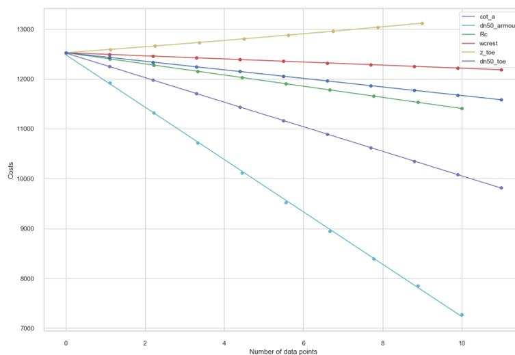
Figure D.11: This figure represent the change in costs per variable, when all other variables are kept constant, each x-axis of the curve is given in table D.19
