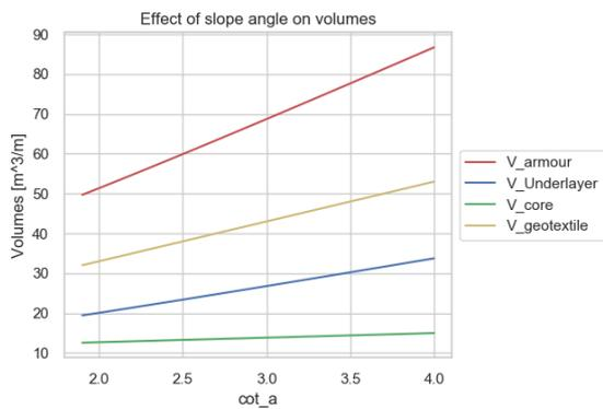
Figure D.12: Change in different volumes for a change in slope angle
