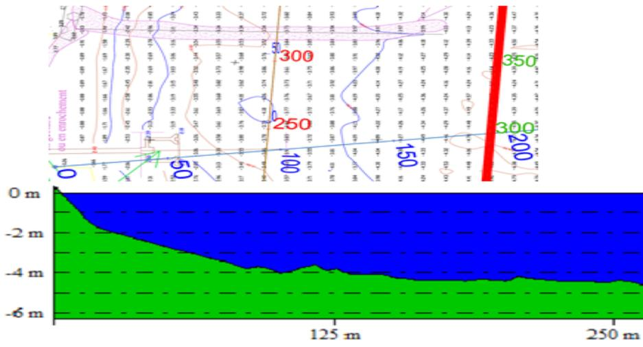
Figure D.3: Bathymetry along the northern breakwater
