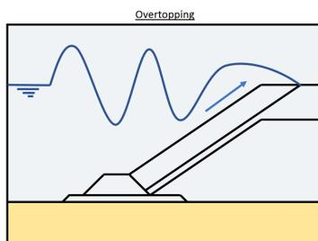
Figure 2.3: Failure Mechanism: Overtopping
