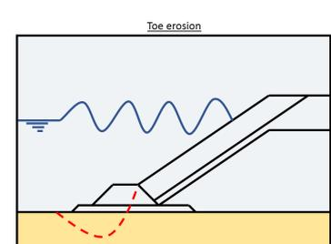
Figure 2.5: Failure Mechanism: Toe erosion
