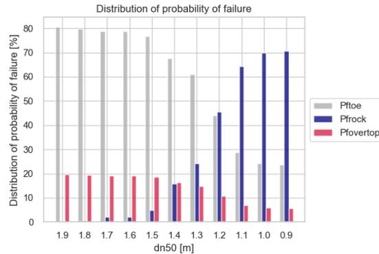
Figure 6.4: Probability of failure distribution of dn50 over failure mechanisms using CMC
