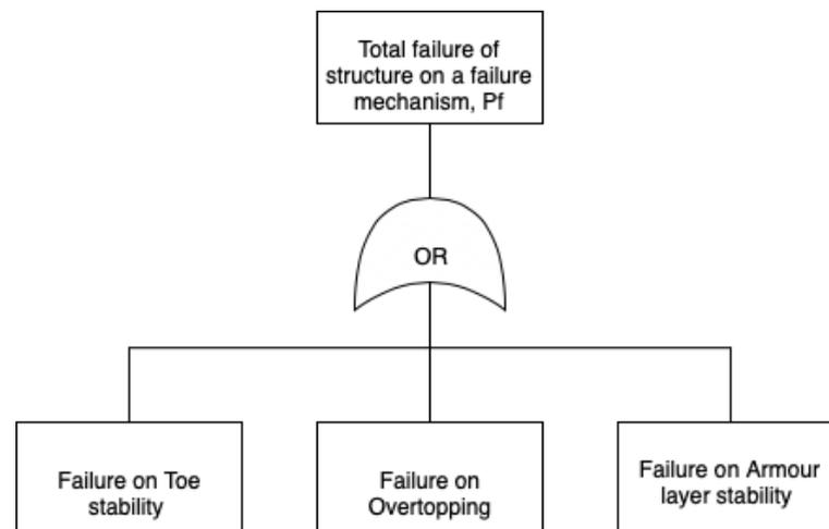
Figure 3.2: Fault tree total probability of failure of system
