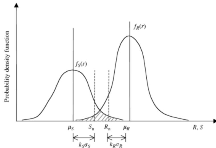
Figure 2.6: Probability density function of resistance and load (Manoj, 2016)
