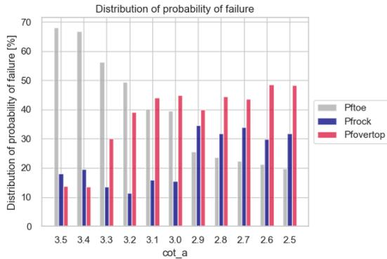
Figure 6.3: Probability of failure distribution of cota over failure mechanisms using CMC
