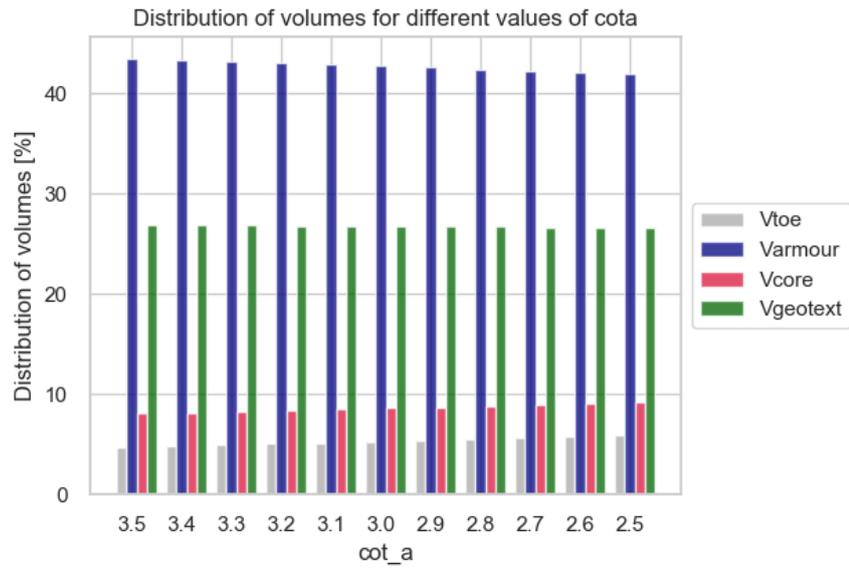
Figure D.14: Change in volume distribution for a change in slope angle
