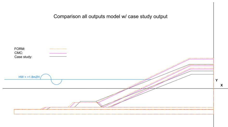
Figure 5.8: Comparison probabilistic cost optimal configurations with case study
