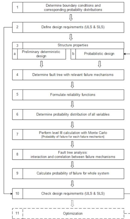
Figure C.1: Full probabilistic design process (Allsop et al., 1999)
