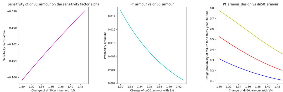
Figure 6.7: Sensitivity of  $dn50_{armour}$  change by 1% to the sensitivity factor  $\alpha$  and probability of failure
