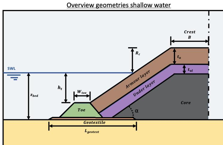
Figure 3.3: An overview of the geometries of the hydraulic structure in shallow water
