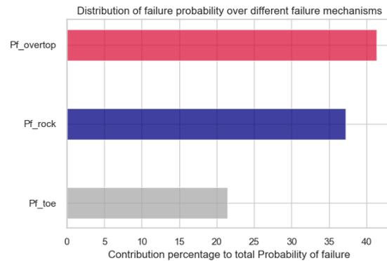
Figure 6.2: Distribution of the probability of failure over different failure mechanisms, comparative combination
