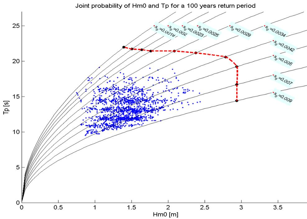
Figure D.7: Joint probability  $H_{m0}$  and  $T_p$  for 100 years return period
