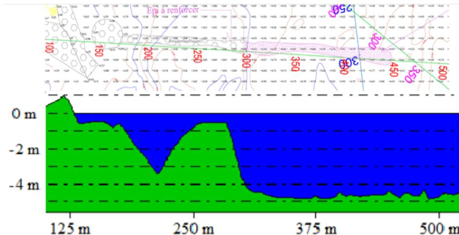
Figure D.2: Bathymetry along the southern breakwater
