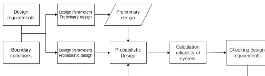
Figure 3.1: Simplified probabilistic design process in the preliminary design phase (Everts, 2016)
