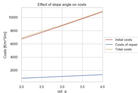
Figure D.13: Change in different costs for a change in slope angle
