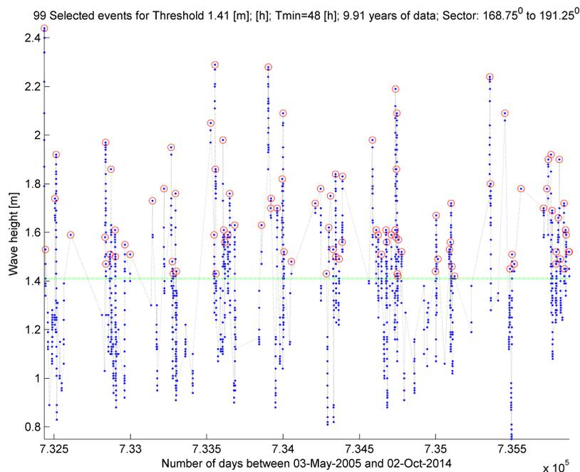
Figure 4.5: POT analysis for significant wave height Extreme observations sample. The red points comprise the extreme observations sample.
