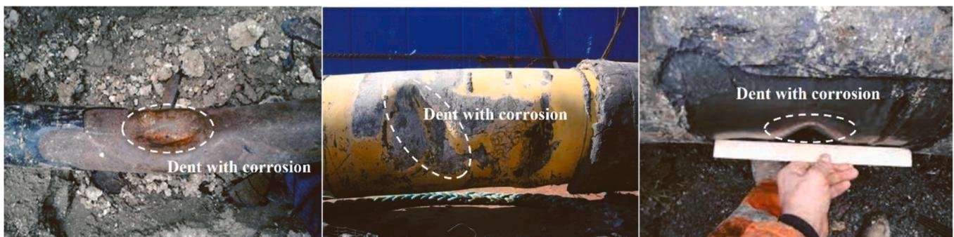
Fig. 2. Dented pipe segment examples with corrosion (Huang et al., 2022a).
