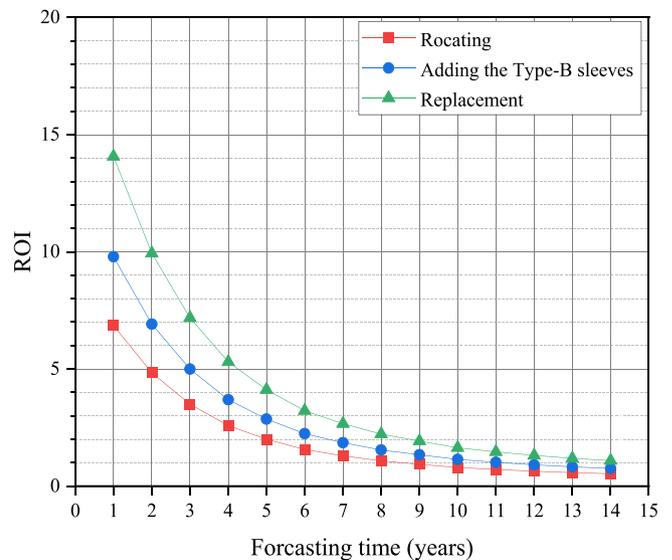
Fig. 17. The ROIs of the three repair measures.
