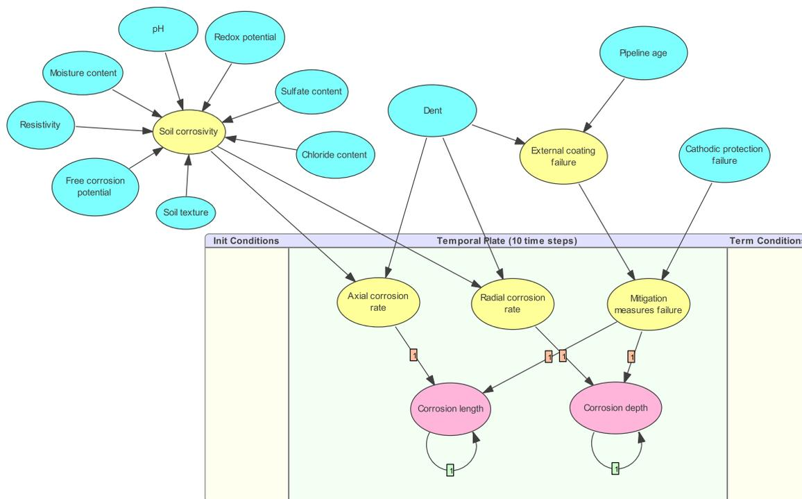
Fig. 5. Developed DBN model for dent-enhanced corrosion.
