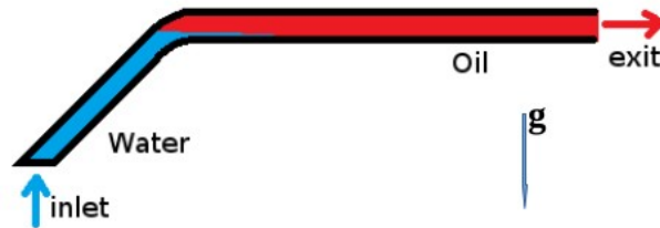
Figure 8.1: Geometry and configuration of the simulated pipe.
