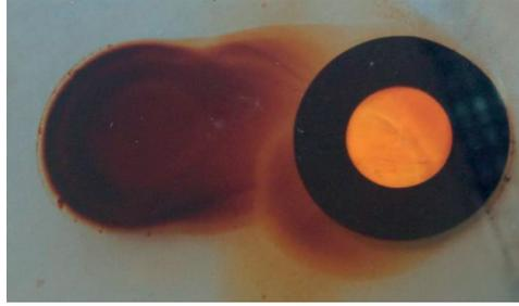
Figure 2.3: Trail formation underneath a glass plate supported by a pocket bearing. Figure from [22].
