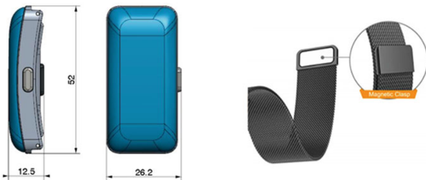
Fig. 4 Wearable wristband dimension and magnetic bracelet closure
