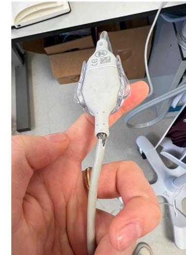
Fig. 22: Cable breakage at the EMC
