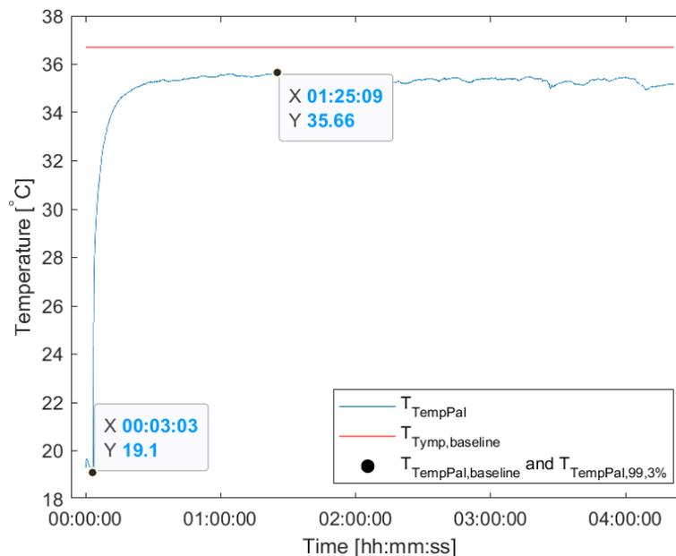
**Figure 6** Temp Pal STP-MB01-1 (iWEECARE Co., Ltd., Taiwan) temperature sensor response time
