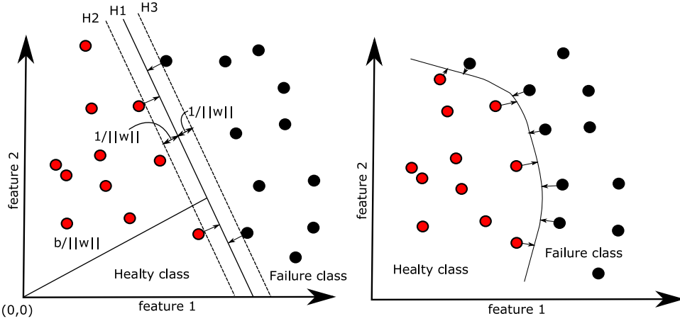
Figure 4.32: Illustration of a linear and a non-linear decision boundary of a one-class support vector machine.
