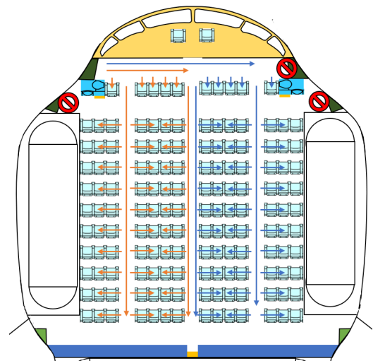
Figure 12.1: Boarding Procedure Schematic, flow of passengers is split into blue and orange at the entrance
