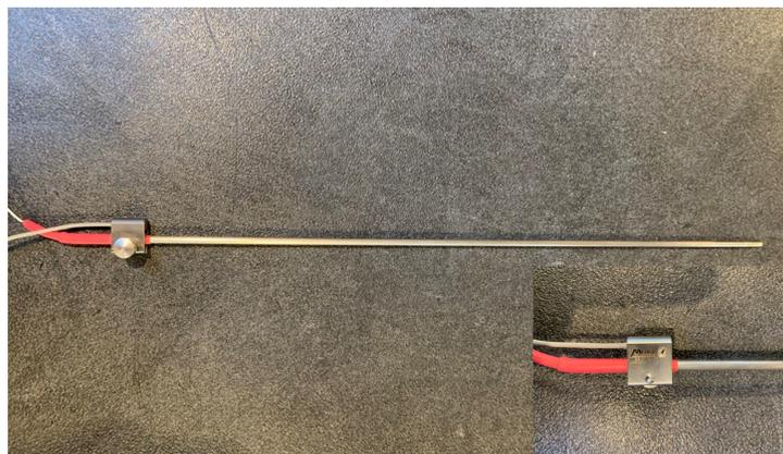
Figure 2.13: Adapter attached on shaft of Laparoscopic Pointer
