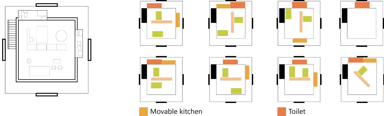
Fig 2. Sky House by Kikutake in 1958 with free plan on the first floor allowing flexible indoor configuration.
