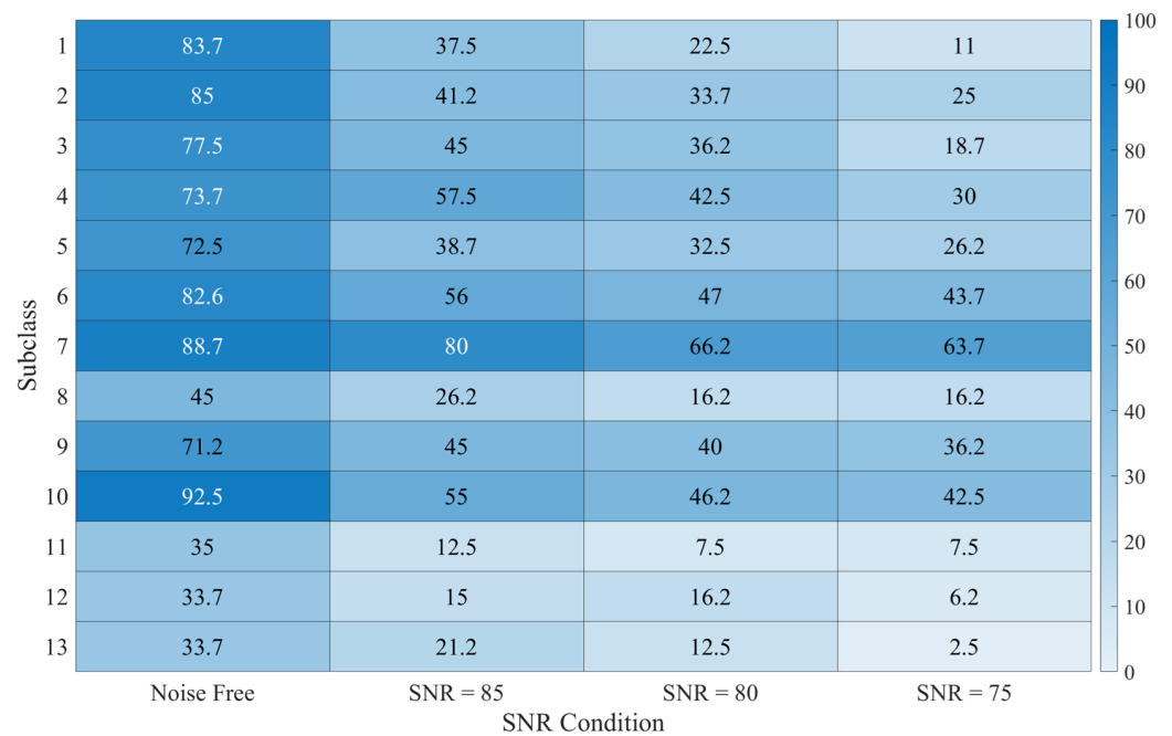
Figure 12. The success rate percentage of the LVQ neural network in the defect detection of the gantry crane system in each subclass.
