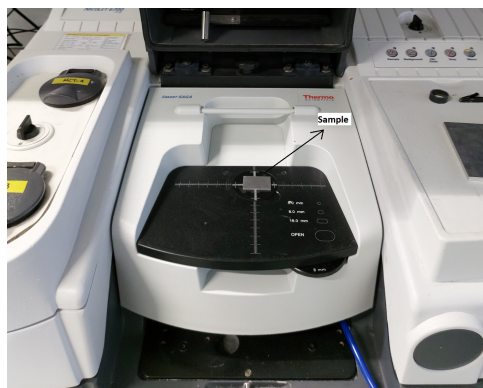
Figure 4.9: Ex-situ FTIR setup of AA2024-T3 exposed to 1mM NaMA placed on the 'Smart SAGA' accessory with exposed surface inverted.
