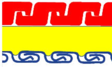
*Figure 2.14: Extrusion of the liner into the adjacent interlocked carcass (Davidson et al., 2016)*
