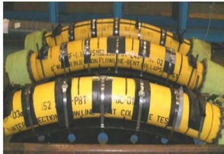
Figure 2.4: Curved collapse test samples (Clevelario et al., 2010)
