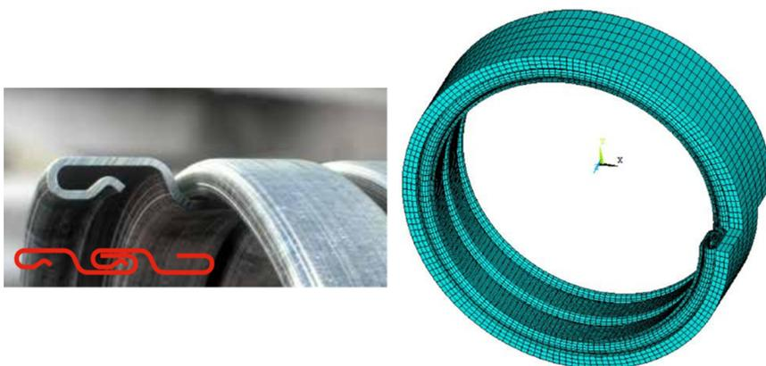
*Figure 2.9: Details of the carcass profile (NOV, 2015) and the 3D full FE model (Gay Neto & Martins, 2012)*
