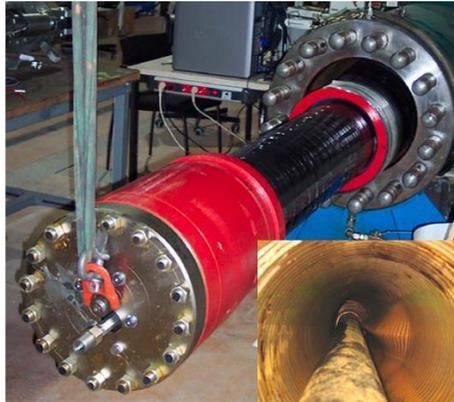
*Figure 2.1: Hyperbaric chamber and end fittings for the collapse test (Miyazaki et al., 2018)*
