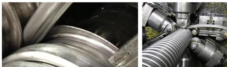
Figure 2.16: Manufacture process of carcass layer (Nielsen, 2014)
