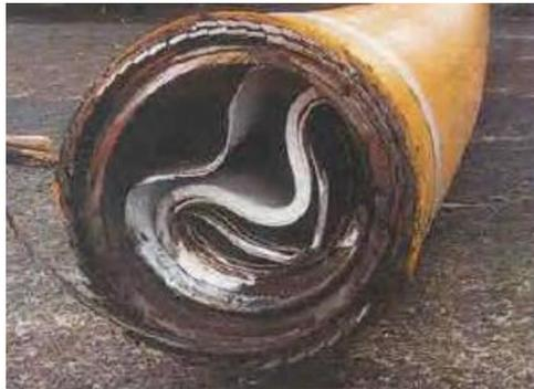
*Figure 1.3: Collapse failure of the flexible riser (Fernando, 2015)*
