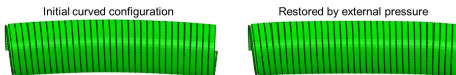
*Figure 5.7: Curved pipe is restored to straight configuration*
