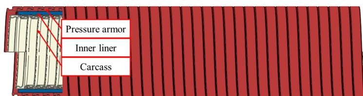
Figure 5.1: Model-A for investigating the wet collapse mechanism of curved flexible risers
