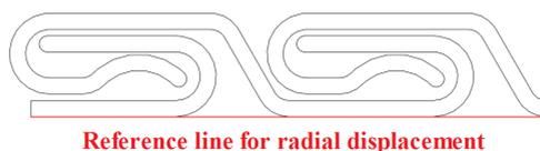
Figure 3.14: Reference line for measuring the radial displacement of FE models
