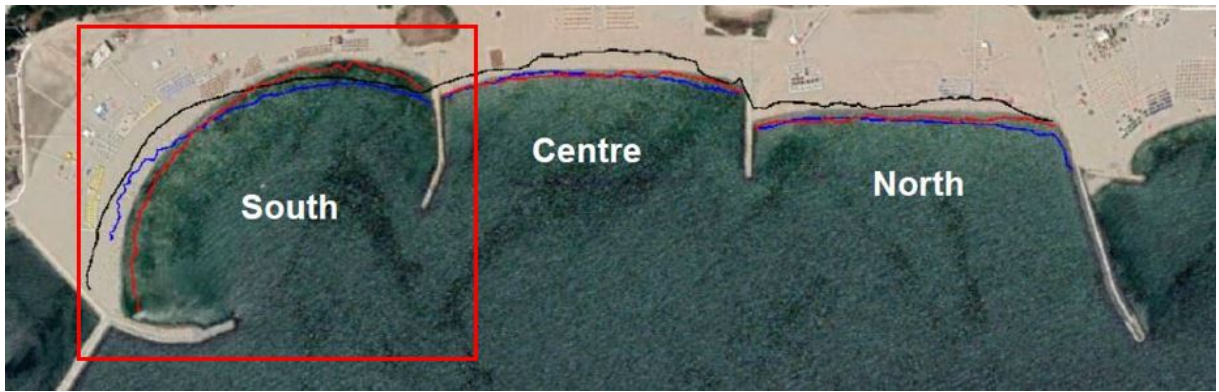
Figure 6.4: Coastlines in 2015 (black), 2016 (blue) and 2020 (red). Red-highlighted coastline section: study area (Brandenburg, 2020)
